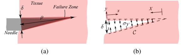
Fig. 2. A schematic of the Strip-Yield zone model. (a) Plastic failure zone with the length of  $\rho$  near the needle tip.  $\delta$  is the CTOD which is approximately equal to the needle outer diameter. (b) The plastic zone is modelled by a compressive stress  $\sigma_Y$  and  $C$  shown by the dashed line is a contour along the boundary of the Strip-Yield plastic zone.
