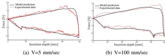
Fig. 9. Model prediction and experimental data for axial force during needle insertion and retraction at velocities of (a) 5 mm/sec and (b) 100 mm/sec.
