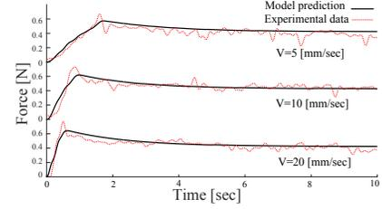
Fig. 5. Results of relaxation tests. Needle force versus time during tissue deformation for velocities of 5, 10, and 20 mm/sec
