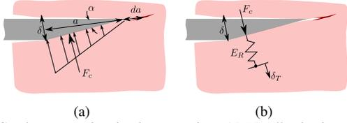
Fig. 3. Crack propagation in tissue cutting. (a) Needle tip-tissue interface during cutting represented by a force distribution with magnitude of  $F_c$ .  $\delta$  is the crack-tip-opening displacement (CTOD),  $a$  is the needle tip length,  $da$  is the incremental crack growth. (b) Modelling finite compliance and viscoelastic behaviour of tissue using a linear solid model element.  $\delta_t = 0$  is the displacement of the tissue sufficiently far from the crack surface.
