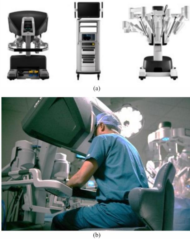
**Fig. 1.** (a) da Vinci Xi Surgical System, (b) the surgeon's console of the da Vinci Xi System [5]. (© [2022] Intuitive Surgical Operations, Inc.)
