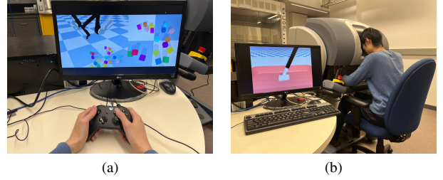
Fig. 4. Experimental setup using teleoperation: (a) ActiveTrack using a joystick controller; (b) GauzeRetrieve using MTM.
