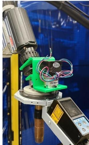
Fig. 4 Profilometer attached behind and along the trajectory of the print path
