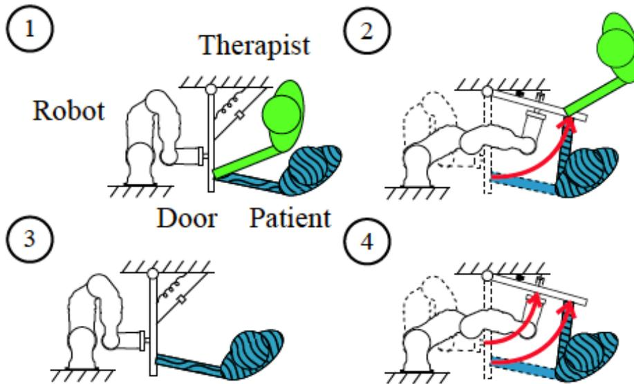
In phases 1 and 2, the therapist provides haptic interaction for the patient when performing a simulated task (in this case opening a door) while the rehabilitation robot observes the intervention through kinesthetic teaching. The LfD algorithm is trained after phase 2. In phases 3 and 4, the robot will imitate the haptic interaction demonstrated by the therapist so as to allow the patient to practice in the absence of the therapist while still receiving haptic guidance.
