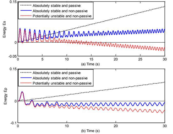
Figure 6. Simulation results for the dual-user teleoperation system. (a) Input energy  $E_s$  at the master #1's port for absolute stability analysis, and (b) passivity observer energy  $E_p$  used for passivity analysis. Simulation parameters are listed in Table I: parameters (A) for the absolutely stable and passive, parameters (B) for the absolutely stable and non-passive, and parameters (C) for the potentially unstable and non-passive.
