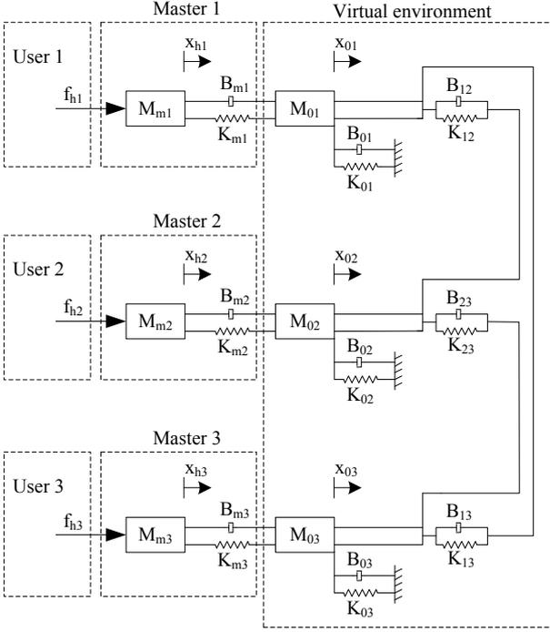
Figure 4. A triple-user collaborative haptic virtual environment system.
