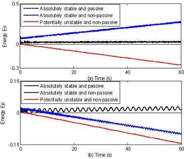
Figure 7. Simulation results for triple-user haptic virtual environment system. (a) Input energy  $E_s$  at the master #1's port for absolute stability analysis, and (b) passivity observer energy  $E_p$  used for passivity analysis. Simulation parameters are listed in Table II: parameters (A) for the absolutely stable and passive, parameters (B) for the absolutely stable and non-passive, and parameters (C) for the potentially unstable and non-passive.
