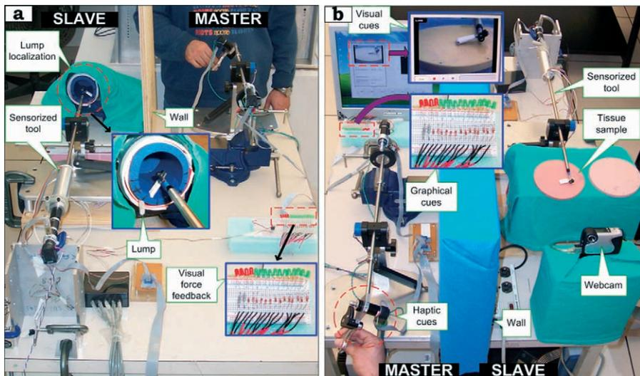
**Fig. 9.5.** Master–slave setup for performing a telemanipulated lump localization and b telemanipulated tissue stiffness discrimination
