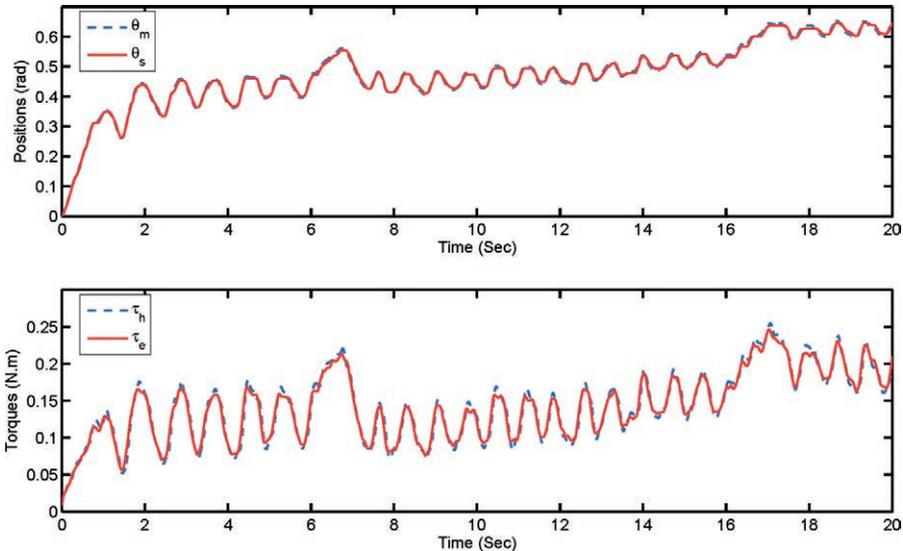
**Fig. 9.3.** Master–slave position and torque, after the slave is in contact with a soft object
