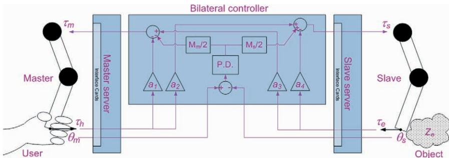
**Fig. 9.2.** Block diagram of four-channel haptic master–slave control
