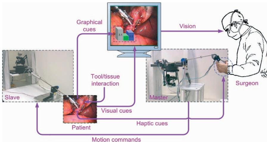
**Fig. 9.4.** Block diagram of master–slave teleoperation with several flows of sensory cues from the slave to the master
