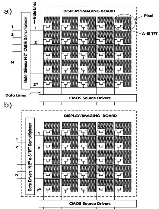
**Fig. 1.** (a) Active matrix arrays with off-board demultiplexer, and (b) active matrix arrays with on-board demultiplexer.
