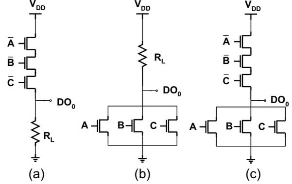
**Fig. 2.** Three different 1:8 demultiplexer circuits in amorphous silicon technology.
