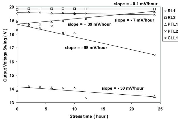
**Fig. 4.** OVSs of different multiplexer circuits as a function of stress time.
