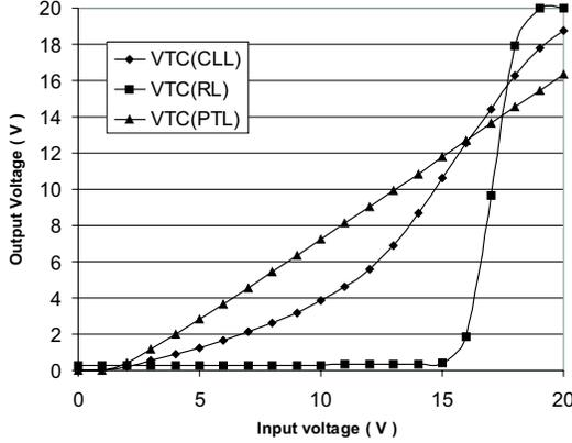
**Fig. 3.** Measured VTCs of the simplified branches of three demultiplexer circuits.
