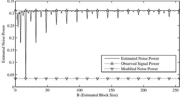
**Fig. 2.** Noise power  $\hat{\sigma}^2(B)$  for JPEG-compressed *Lena* with a block size of 16, the power in the observed signal  $\mathbf{d}_p$ , and the modified noise power. Each triangle mark corresponds to a multiple of 16.
