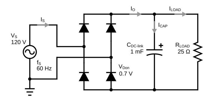
Parameters:  $V_S = 120$ V,  $f_S = 60$ Hz, C = 1mF,  $R_{LOAD} = 25\Omega$ ,  $V_{Don} = 0.7$ V
