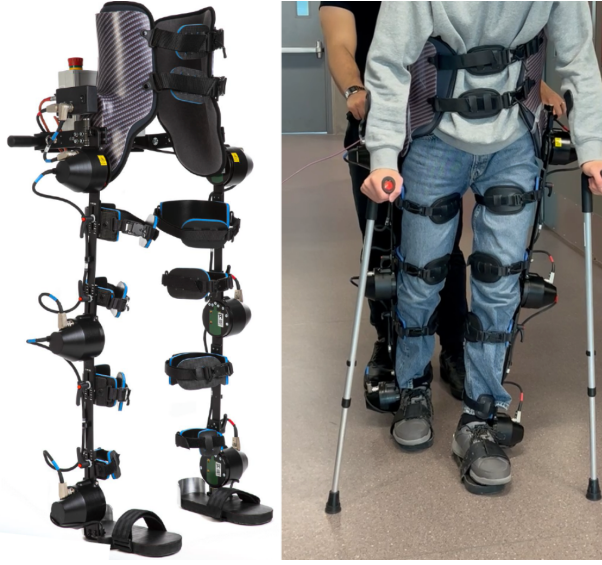
Fig. 1. The Exo-H3 Exoskeleton, a lower limb wearable robotic exoskeleton device designed by Technaid S.L.
