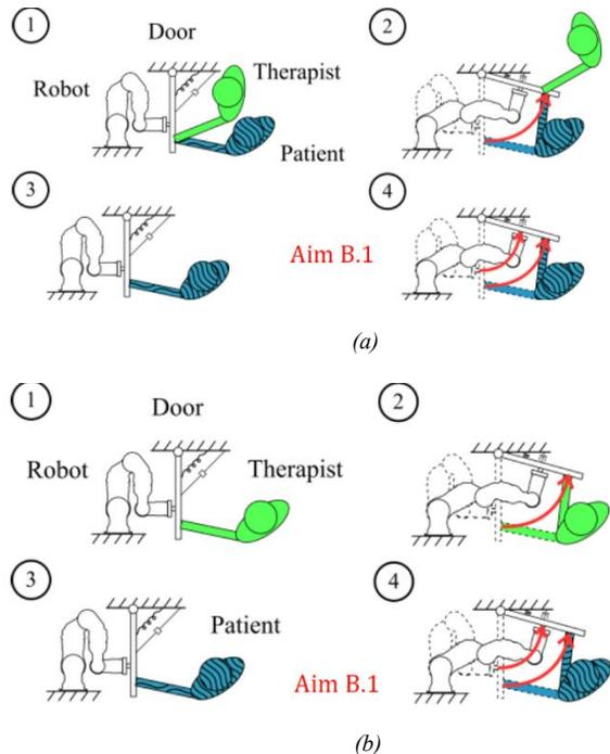
Figure 1: Top figure (a) shows the first way to implement the tasks. The therapist and the patient are working together during the demonstration phase. Later in the reproduction phase, the patient works alone with the robot. Bottom figure shows a second way to implement the task. First the therapist works alone in the demonstration phase. Later in the reproduction phase, the patient works alone with the robot.
