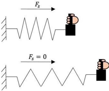
Figure 3: This figure shows the force task. The virtual spring is attached to the robot's end-effector and it applies a force  $F_s$  to the user. The top figure shows the initial position at the beginning of the task, here the spring is compressed and it is applying force to the user, while the bottom figure shows the therapist's learned behavior, the goal is to decompress the spring until  $F_s$  becomes equal to zero.
