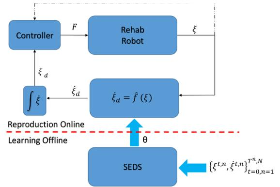
Figure 4: Block diagram showing the learning and reproduction phases
