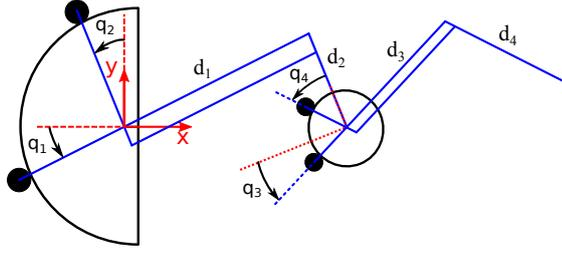
Fig. 3. Schematic of the four DoF master robot
