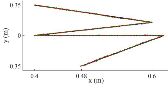
Fig. 9. Reference (Solid black line), Scenario 1 (Blue Dashed line), Scenario 2 (Red Dashed-dot line), and Scenario 3 (green dot line) paths of user #3 for trajectory following task.
