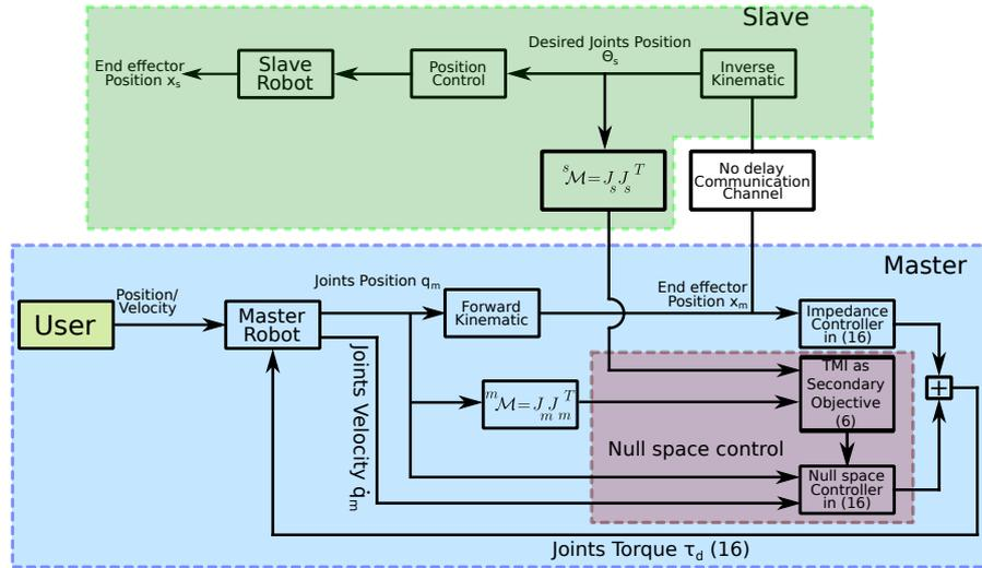
Fig. 4. Block diagram of the unilateral teleoperation system.
