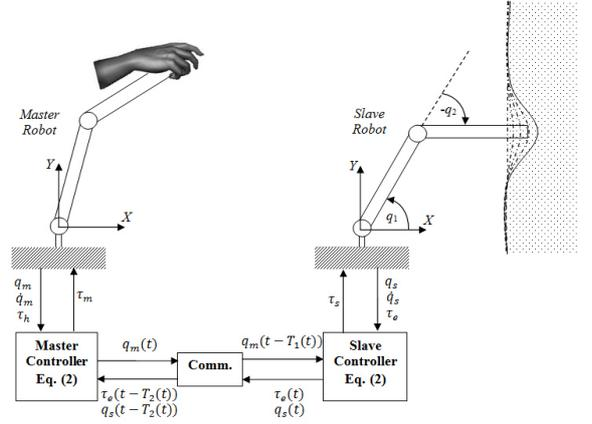
Figure 1. Block diagram and signal flows of the proposed telerobotic system.
