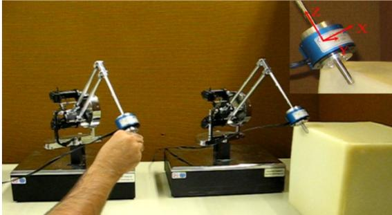
Figure 9. Experimental setup consisting of two PHANTOM Premium 1.5A's and the force sensor frame.
