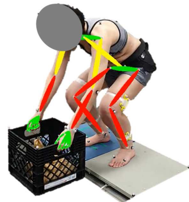
Figure 2. Skeletal model captured by the markerless motion capture system during the lifting motion.
