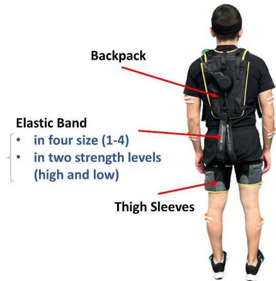
Fig. 1. Apex exoskeleton. There are eight configurations of the elastic bands as a combination of four sizes (1-4) and two strength levels (low and high).
