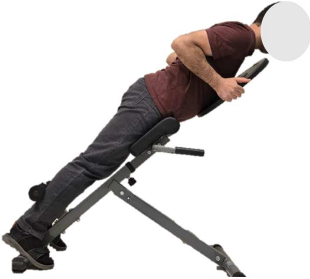
Fig. 2. Endurance time test. Hip is supported at the edge of the bench, and the participant holds a 5 kg weight in their hands close to the chest.
