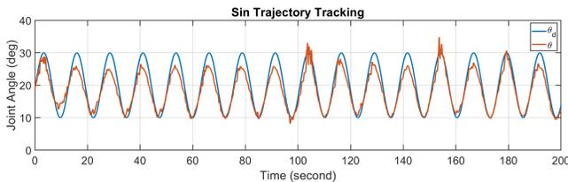
Fig. 5. Sin trajectory tracking using dynamic torque allocation
