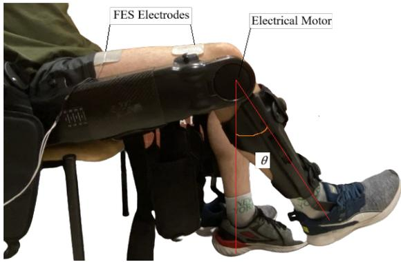
Fig. 2. Experimental set-up of hybrid FES-Exoskeleton
