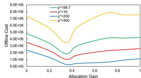
Fig. 3. Offline cost function is plotted for different  $p^*$  values. As it is shown the best cost function in terms of convexity and having a global minimum point at  $x_d = 0.35$  is the one with  $p^* = 99.7$
