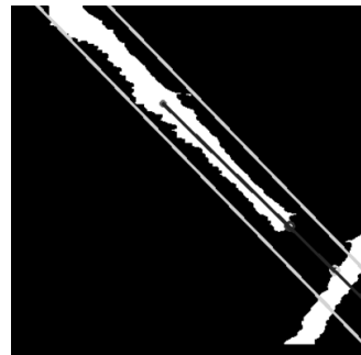
Fig. 5. The result of the image processing required to find the surgical tool shaft and tip. The green lines form the boundary of the ROI, the purple line identifies the surgical tool shaft, and the blue dot shows the surgical tool tip.
