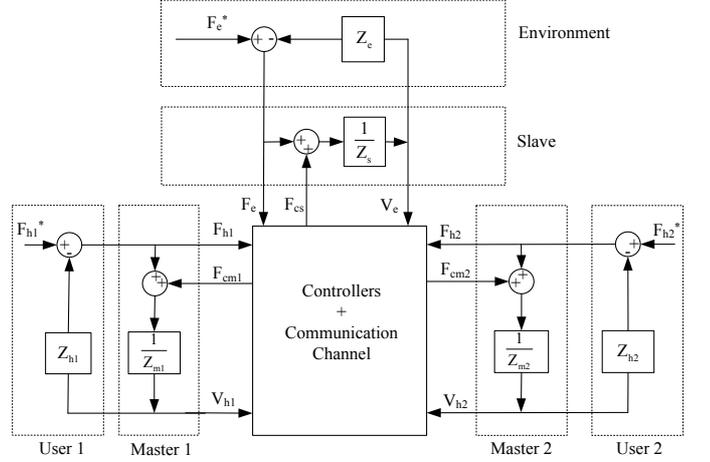
Figure 3. A dual-user haptic teleoperation system under four-channel control.
