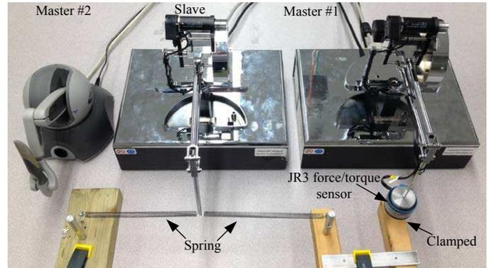
Figure 8. Experimental setup where the master #2 is connected via passive spring to stiff wall, the slave is in free motion. In absolute stability experiment, the master #1 is controlled by a human user. In passivity experiment, the master #1 is physically clamped.
