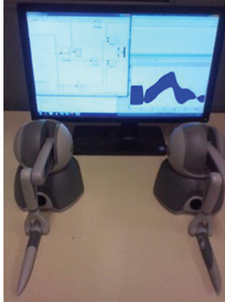
Figure 17: Two PHANToM robots connected to the teleoperation system.
