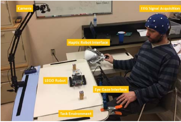
Fig. 2 Picture of the system with the human-robot interface and the task environment.
