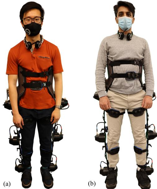
Fig. 5. Exo-H3 lower limb exoskeleton worn by two able-bodied users for walking. The participants use a wireless headset to command the exoskeleton. (a) User 1 (21-year-old) and (b) User 2 (33-year-old).
