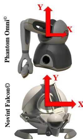
(b) The coordination frames assigned to the Novint Falcons<sup>®</sup> and Phantom Omni<sup>®</sup>.
