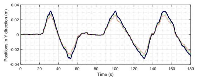
(c) Operator positions of SMT in Y direction with respect to time.
