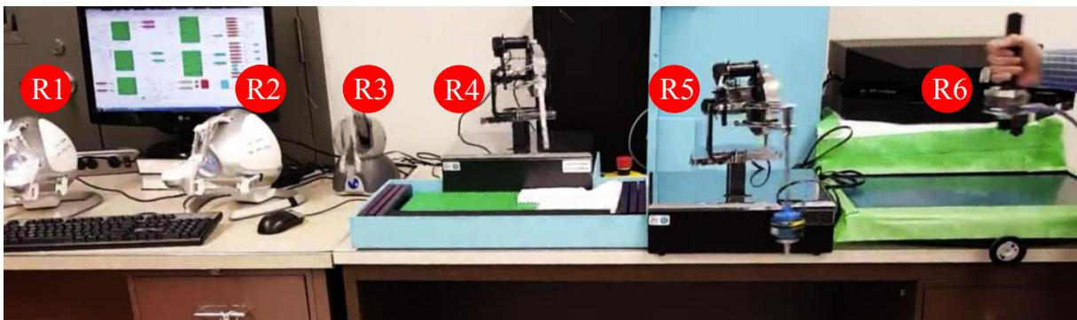
**Figure 12.** In this figure, six non-homogeneous robots participate in a rehabilitation process as discussed in Fig. 11. A dual set of Novint Falcon<sup>®</sup>, one Phantom Omni<sup>®</sup>, Two Phantom Premium<sup>®</sup> robots, and one Quanser<sup>®</sup> robot participate in the process, forming R1 to R6, respectively.
