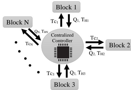
**Figure 1.** Centralized Controller. Each block sends its position and sensed force to the central controller. The central controller calculates the control torque using (8) and sends its associated part to each individual block (i.e.  $\{T_{C1}, \dots, T_{CN}\}$ ). As a drawback of the centralized controller, it is clear that if the centralized controller is damaged, the whole system will fail.
