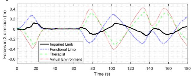
(d) Operator sensed forces of SMT in X direction with respect to time.
