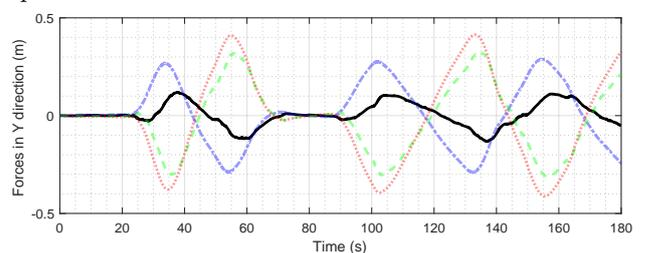
(e) Operator sensed forces of SMT in Y direction with respect to time.
