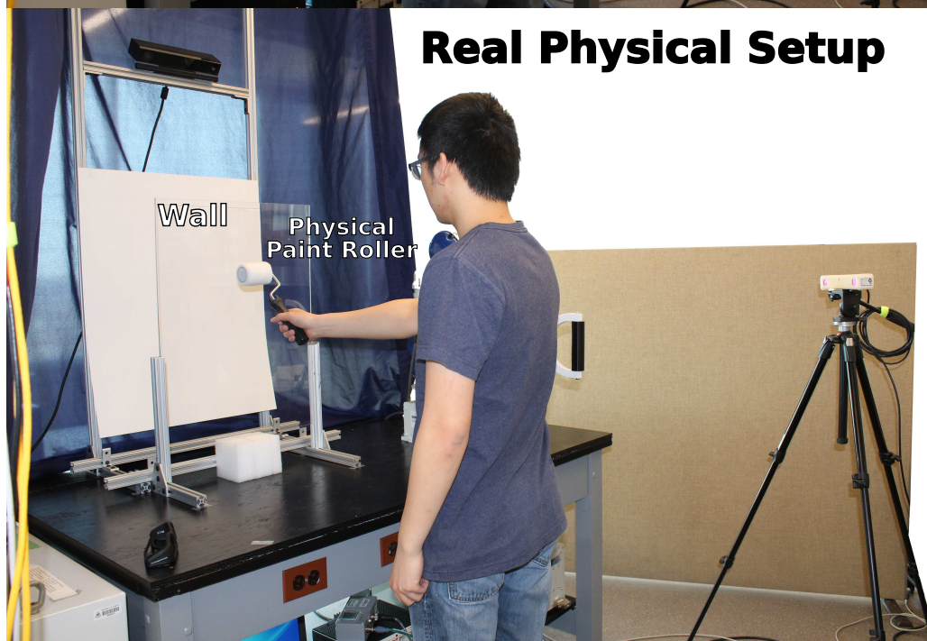
Figure 7.2: Painting task experimental setup for the robot-AR condition (top) and the real-life equivalent condition (bottom). The projector is not shown. Through AR, the paint roller will pop out in 3D from the perspective of the user in a geometrically correct position and orientation relative to the robot end-effector.
