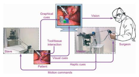
**Fig. 9.4.** Block diagram of master-slave teleoperation with several flows of sensory cues from the slave to the master
