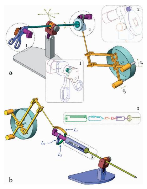
Fig. 9.1. a Haptic HMI (master), and b sensorized robot (slave) suitable for a minimally invasive environment
