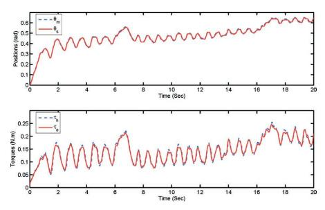
Fig. 9.3. Master-slave position and torque, after the slave is in contact with a soft object
