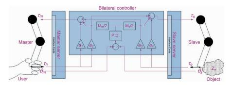
Fig. 9.2. Block diagram of four-channel haptic master-slave control
