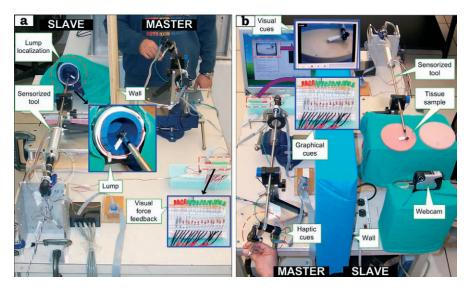
**Fig. 9.5.** Master–slave setup for performing **a** telemanipulated lump localization and **b** telemanipulated tissue stiffness discrimination
