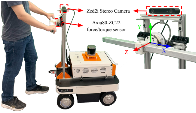
Fig. 1: (left) Illustration of mobility assistance with the Smart Walker - (right) Coordinate reference frame on the force/torque sensor
