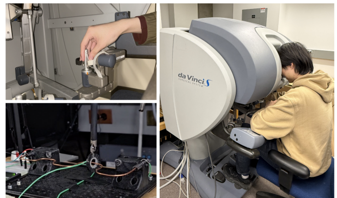
Figure 1: Ring-and-rail task for training/assessing fundamental surgical skill. The operator teleoperates the PSM to guide a rigid ring along a narrow, curved metal wire without making contact. This surgical training task simulates critical aspects of real surgical procedures, such as hand-eye coordination, fine motor control, spatial planning, and operation within constrained environments.
