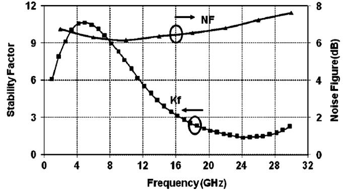
Fig. 13. Measured noise figure of fabricated NCDA and stability K-factor extracted from measured S-parameters.
