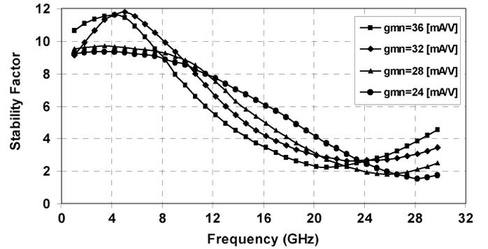
Fig. 10. Simulated stability K-factor for different values of  $g_{mn}$ .
