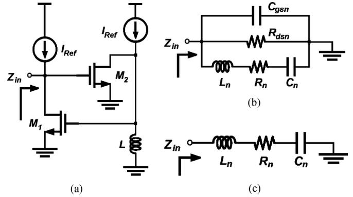
Fig. 2. Negative capacitance cell. (a) Simplified circuit schematic. (b) Small-signal equivalent circuit. (c) Simplified equivalent circuit.
