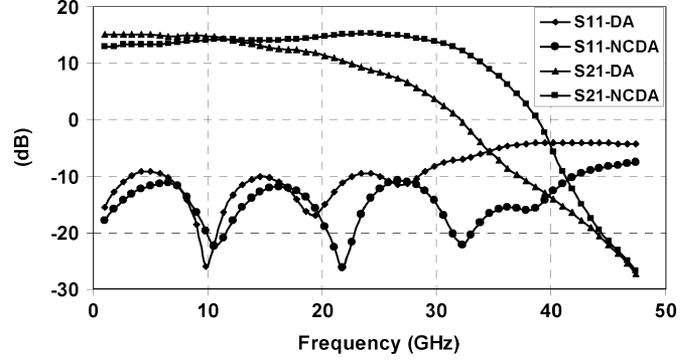
Fig. 8. Comparison of gain and bandwidth for six-stage NCDA and conventional DA.
