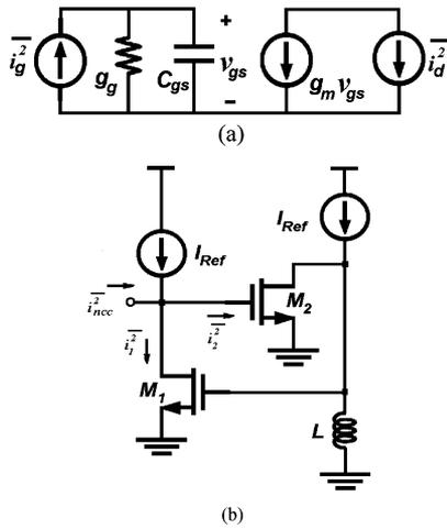
Fig. 14. Noise modeling. (a) Gate noise model. (b) Negative capacitance noise current model.
