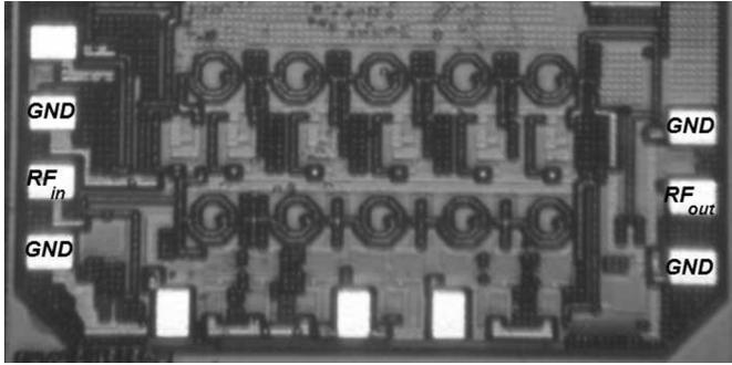
Fig. 11. Die photograph for implemented six-stage NCDA.
