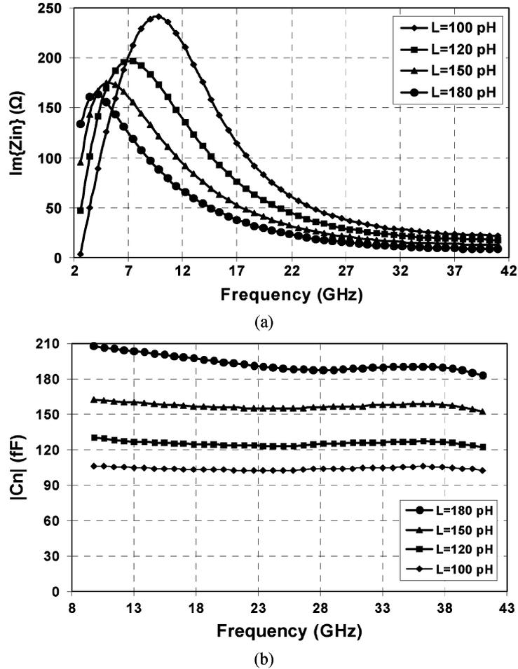
Fig. 3. Simulated curves of  $Z_{in}$  in terms of frequency for  $g_{mn}^2 = 1 \text{ mA/V}^2$  and different values of the inductor. (a) Imaginary component of  $Z_{in}$ . (b) Absolute values of the negative capacitance.
