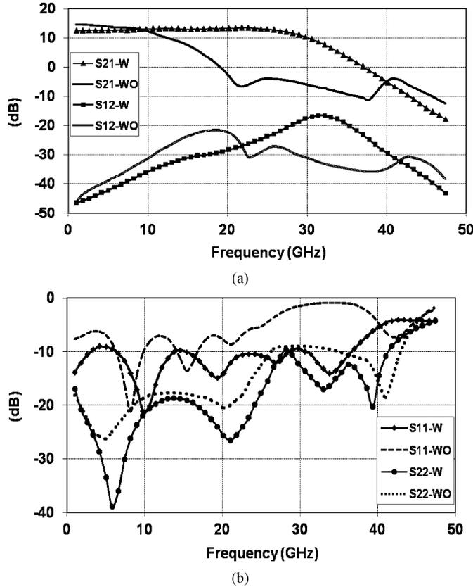
Fig. 12. Measured S-parameters of implemented NCDA without activated negative capacitance network (WO) and with activated negative capacitance (W) (a)  $S_{21}$  and  $S_{12}$  (b)  $S_{11}$  and  $S_{22}$ .
