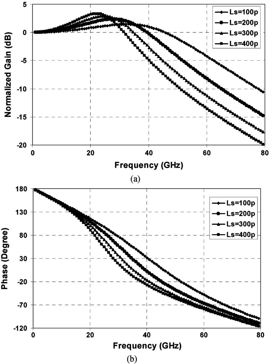
Fig. 5. Simulated frequency response of series-peaking network at the cascode node for different values of the inductor (a) gain response (b) phase response.
