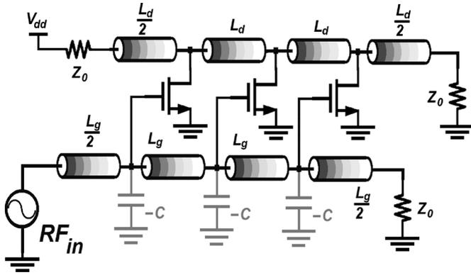
Fig. 1. Conventional DA structure with adding negative capacitance on the gate transmission line.
