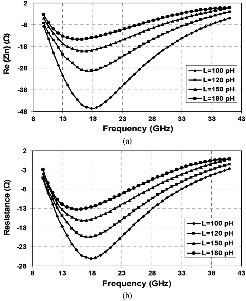
Fig. 4. Simulated curves of  $Z_{in}$  in terms of frequency for  $g_{mn}^2 = 1 \text{ mA/V}^2$  and different values of inductor. (a) Real component of  $Z_{in}$ . (b) Extracted values of negative resistance.
