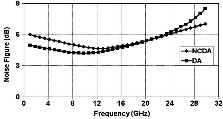
Fig. 9. Comparison of simulated noise-figure for six-stage NCDA and conventional DA.
