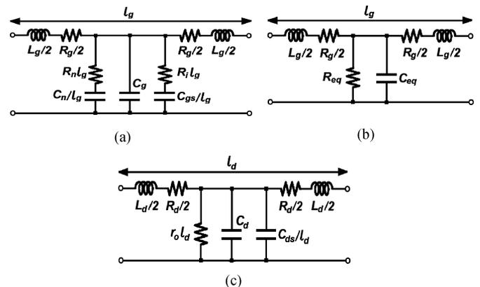
Fig. 7. Equivalent small-signal model of the DA transmission lines (TLs). (a) Equivalent circuit for the gate TL. (b) Series-to-parallel impedance transformation in equivalent circuit. (c) Equivalent circuit for the drain TL.
