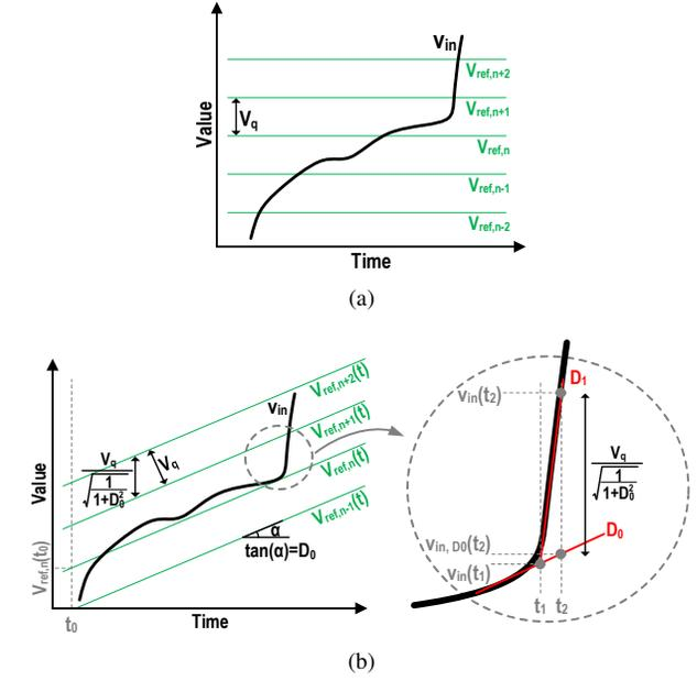
Fig. 3. Reference levels in (a) conventional LC, and (b) MDLC schemes.
