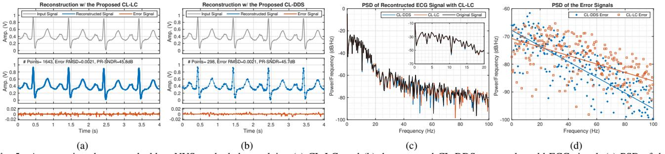
Fig. 5. A comparison between clockless NUS methods by applying (a) CL-LC, and (b) the proposed CL-DDS on a real-world ECG signal, (c) PSD of the reconstructed ECG signals by CL-LC and CL-DDS, and (d) PSD of error signals after reconstruction of ECG signal.
