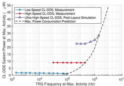
Fig. 13. Maximum power dissipation of the CL-DDS system vs. TRG frequency at the maximum activity of the system.
