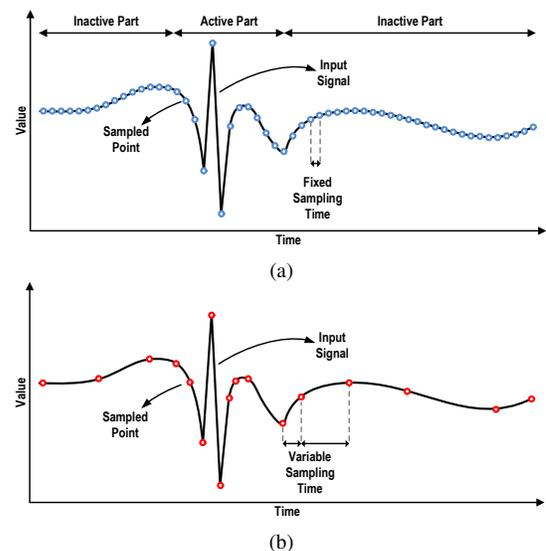
Fig. 1. Sampling a signal by (a) uniform, and (b) non-uniform method.
