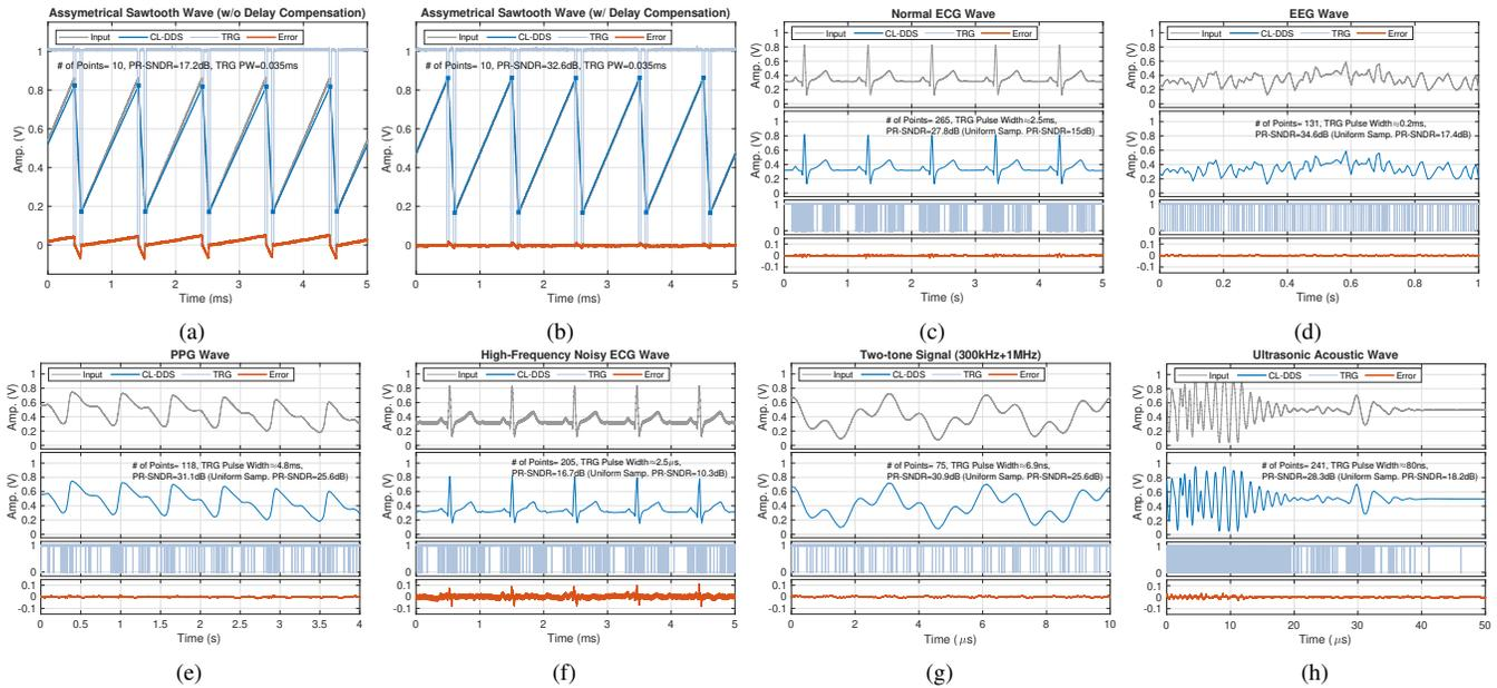
Fig. 12. Measurement of system responses to a saw-tooth signal (a) without a compensation delay, and (b) with a compensation delay. Experimental results of the proposed low-speed CL-DDS system for (c) normal ECG, (d) EEG, (e) PPG, and (f) high-frequency noisy ECG. Experimental results of the proposed high-speed CL-DDS system for (g) two-tone signal, and (h) Ultrasonic signal.
