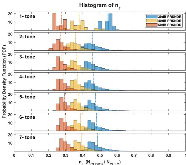
Fig. 6. Distribution of  $n_r$  for different tones and multiple targeted PR-SNDR values for 2000 iterations.
