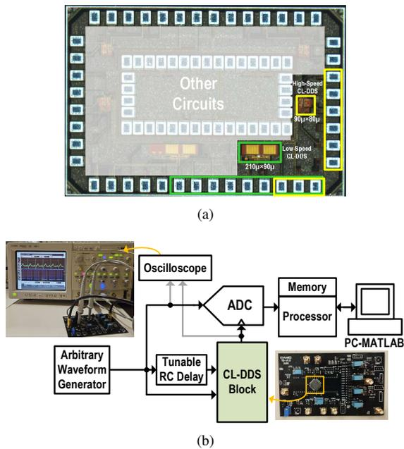
Fig. 11. (a) Die micrograph of the proposed CL-DDS, and (b) test-bench.
