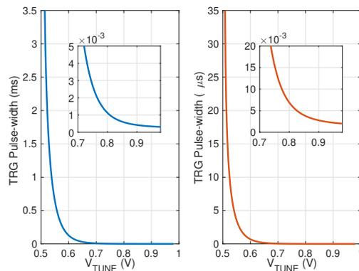
Fig. 10. Tuning the width of output TRG pulse by  $V_{tune}$  in the proposed low- and high-speed design of monostable circuit.
