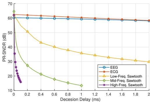
Fig. 9. The effect of decision delay on the quality of reconstruction for various signals with different frequency contents.
