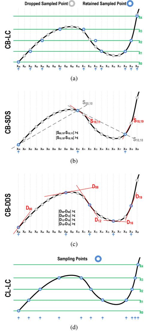
Fig. 2. Detection of significant events in an arbitrary signal by three NUS schemes: (a) CB-LC, (b) CB-SDS, (c) CB-DDS, and (d) CL-LC.
