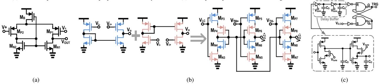
Fig. 8. Circuit implementation of (a) the main amplifiers, (b) the window comparator, and (c) the monostable.
