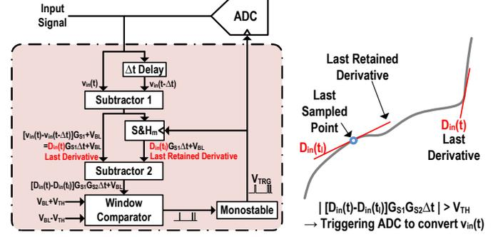
Fig. 4. Overall block diagram of the CL-DDS scheme.
