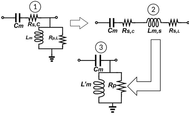
Fig. 4. Impedance matching network series-to-parallel and parallel-to-series transformation.
