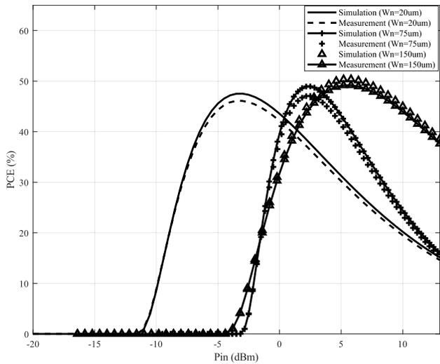
Fig. 12. Comparison of simulated and measured efficiency for the proposed harvesters at various input power levels ( $V_o = 1V$ ).
