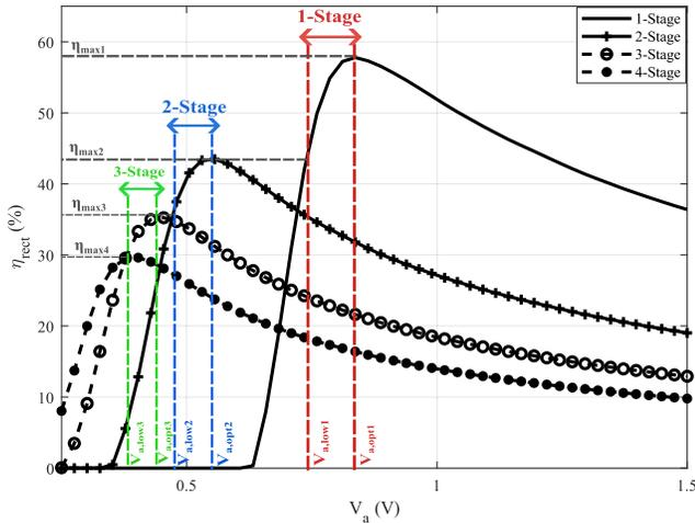
Fig. 8. Maximum achievable efficiency for different number of stages ( $V_o = 1V$ ).
