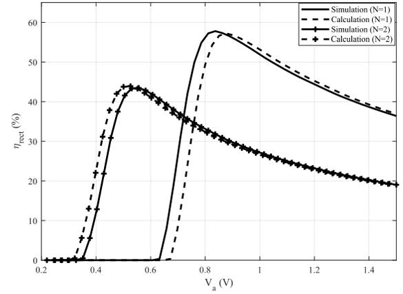
Fig. 6. Rectifier efficiency as a function of its input voltage amplitude for  $N=1$  and  $N=2$  ( $V_o=1V$ ).
