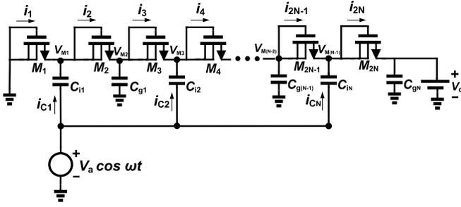
Fig. 13. An N-Stage rectifier loaded by a voltage source.
