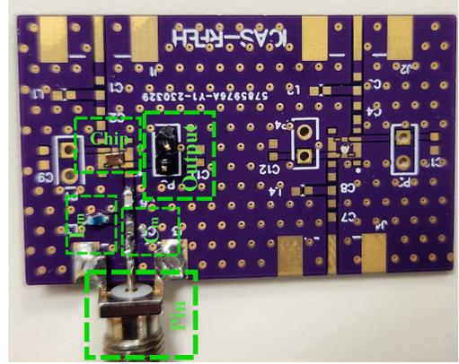
Fig. 11. Proposed PCB setup for experimental verification.
