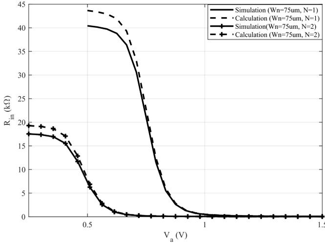
Fig. 7. Rectifier input resistance as a function of input voltage amplitude for  $N = 1$  and  $N = 2$ . ( $V_o = 1V$ ,  $W_n = 75\mu m$ ).
