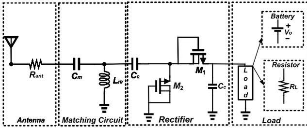
Fig. 1. RF energy harvester schematic.
