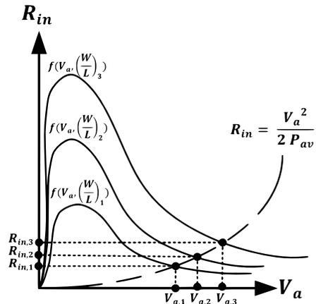
Fig. 3. Rectifier optimal operation point.
