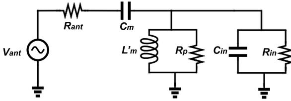
Fig. 5. An RF energy harvester model with a lossy matching network.
