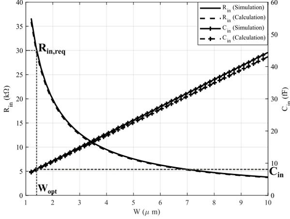
Fig. 9. Rectifier input resistance and capacitor as function of devices' width (prepared for  $V_a = 0.975$  V,  $N=1$  and  $V_o = 1$  V).
