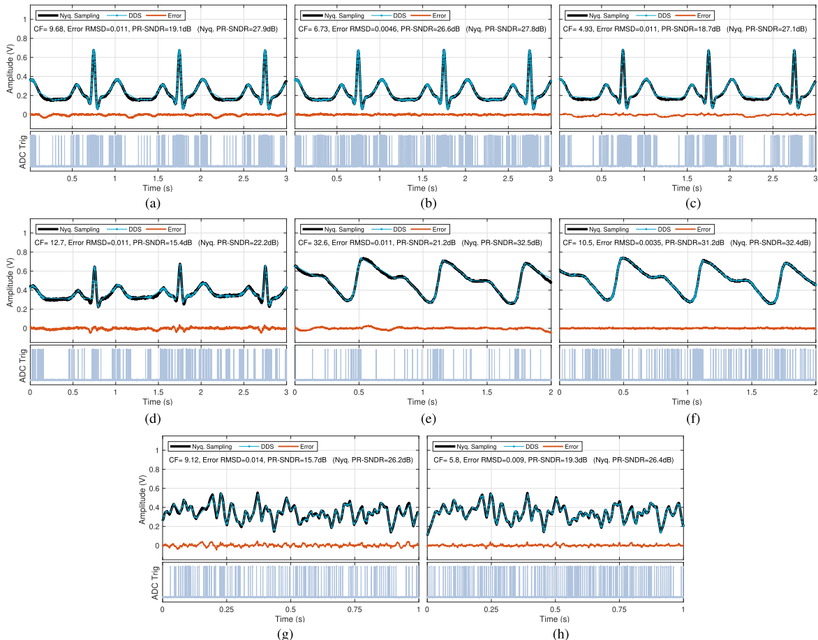
Fig. 17. Experimental results of the DDS system, (a) ECG signal with high CF setup and a 1 kHz clock, (b) ECG signal with low CF setup and a 1 kHz clock, (c) ECG signal with 250 Hz clock, (d) Noisy ECG signal with high CF setup and a 1 kHz clock, (e) PPG signal with high CF setup, (f) PPG signal with low CF setup, (g) EEG signal with high CF setup, and (h) EEG signal with low CF setup.
