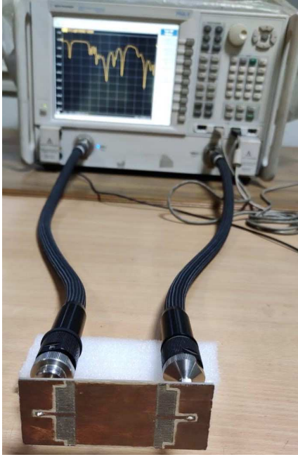
Fig. 6. The back-to-back transitions with VNA.
