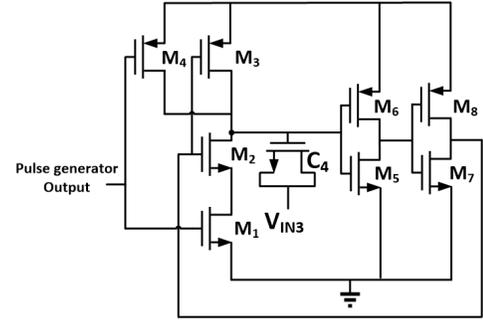
Fig. 10. Carrier oscillator.
