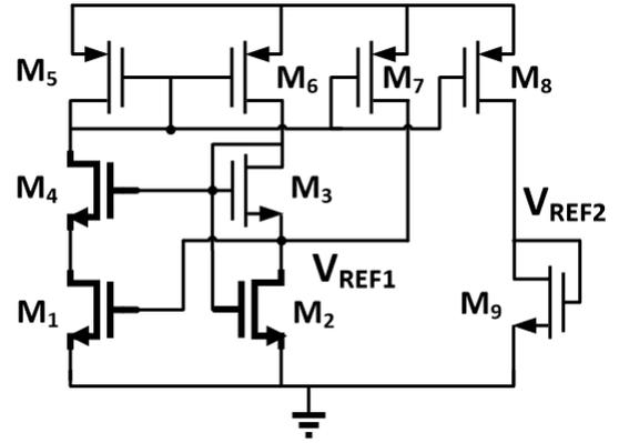
Fig. 8. Reference voltage generator.
