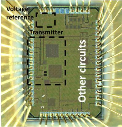
Fig. 16. Chip microphotograph.
