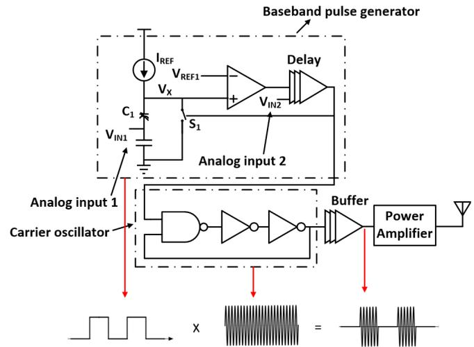
Fig. 2. Proposed ultra-low-power transmitter.
