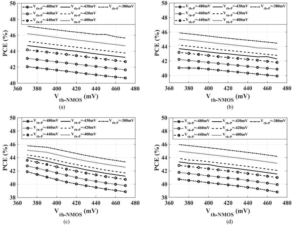
Fig. 8. Simulation of PCE versus NMOS and PMOS threshold voltage variation for (a) implementation I, (b) implementation II (V1), (c) Implementation II (V2), and (d) implementation III with applied input power of  $-15$  dBm and connected output load of  $1M\Omega$ .
