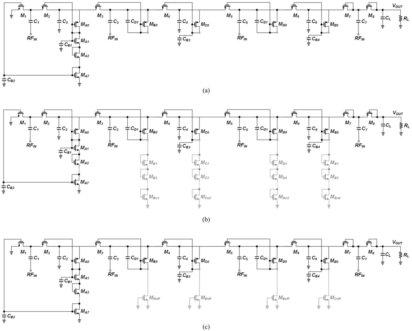
Fig. 6. Proposed single-ended self-compensated RF energy harvester using three implementations for the high impedance path, (a) Implementation I, (b) Implementation II (V1) and (V2), and (c) Implementation III.
