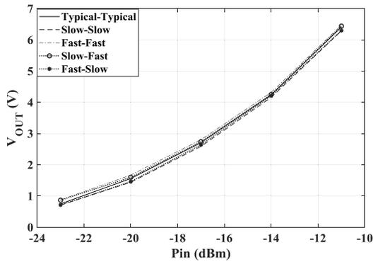
Fig. 9. Simulation of output voltage versus input power for different process corners of Implementation I when the rectifier is connected to  $1M\Omega$  load.
