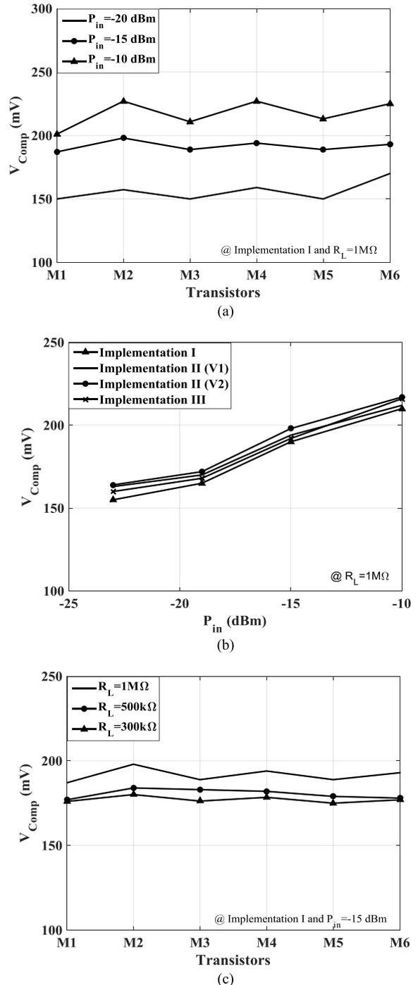
Fig. 7. (a) Generated compensation voltage for each transistor at different input power levels for implementation I, (b) compensation voltage versus input power for all implementations, (c) generated compensation voltage for each transistor at different output loads for implementation I.
