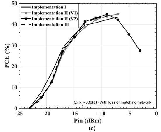
Fig. 11. PCE as the function of input power for a)  $1\text{M}\Omega$ , b)  $500\text{k}\Omega$  and c)  $300\text{k}\Omega$  loads, without considering the loss of the matching network.
