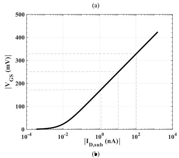
Fig. 5. (a) Employed auxiliary transistor for producing the desired compensation voltage. (b) Gate-source voltage drop as the function of leakage current.
