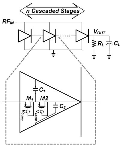
Fig. 3. Simulated circuit for finding the optimum compensation voltage and the optimum number of stages.
