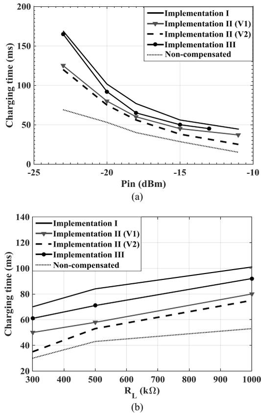
Fig. 15. Measured 10-90% charging time for different implementations (a) versus  $P_{in}$  for  $R_L = 1M\Omega$  and  $C_L = 47nF$ , (b) versus  $R_L$  for  $P_{in} = -20dBm$  and  $C_L = 47nF$ .
