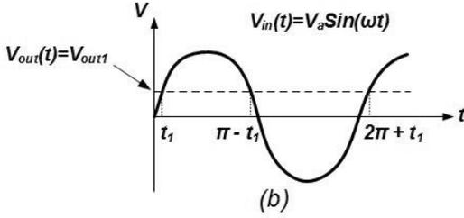
Fig. 1. (a) Schematic of threshold-compensated, single-transistor rectifier. (b) Input and output voltage waveforms of a single-transistor rectifier.
