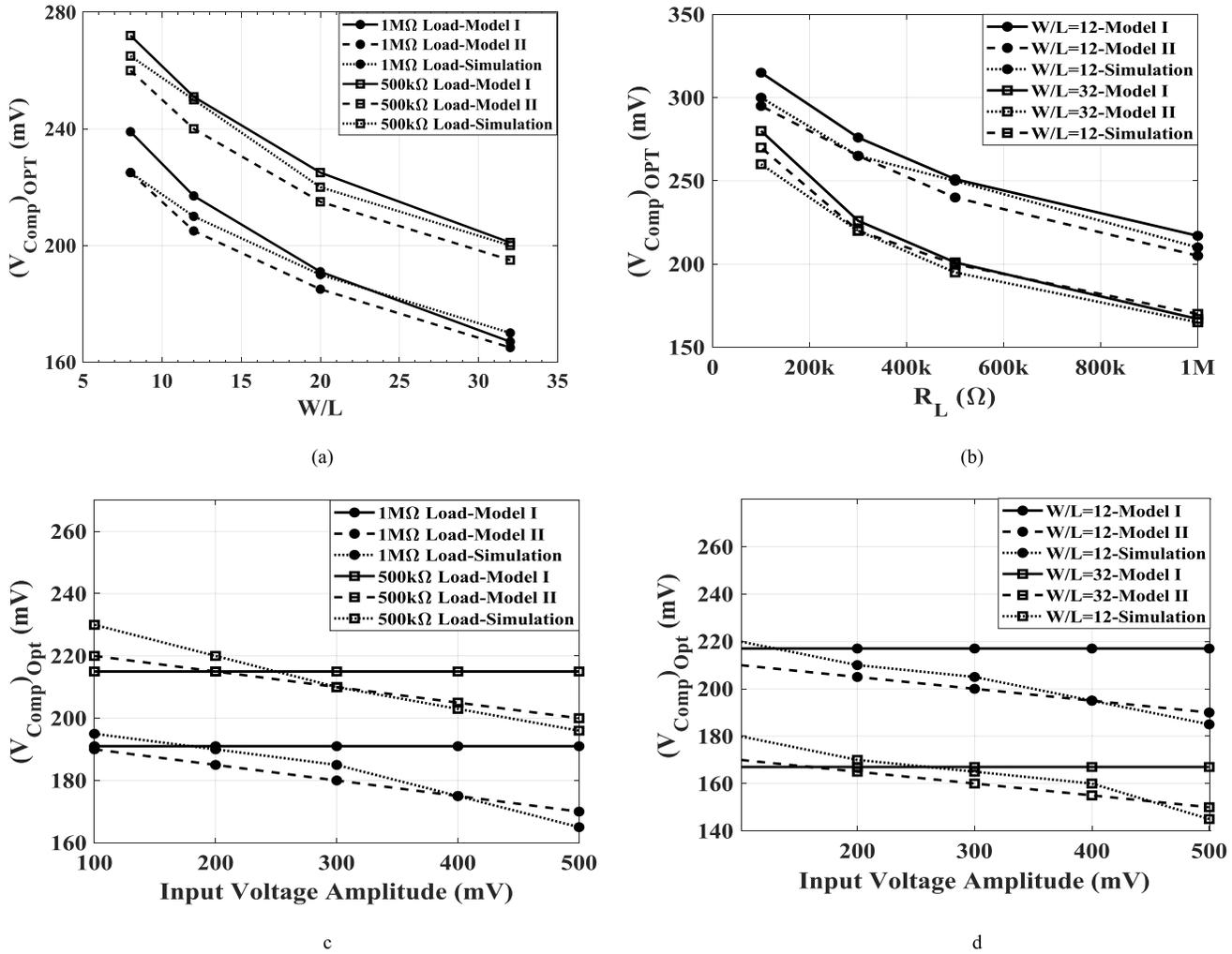
Fig. 2. Optimum compensation voltage for having maximum PCE versus (a) size of transistor ( $W/L$ ) for different load resistances and fixed input voltage amplitude of 200 mV, (b) load resistance ( $R_L$ ) for different size of transistor and fixed input voltage amplitude of 200 mV, (c) input voltage amplitude for different size of transistor ( $W/L$ ) and fixed load resistance of  $1M\Omega$ , and (d) input voltage amplitude for different load resistances and fixed  $W/L$  of 20.
