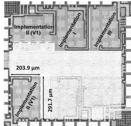
Fig. 10. Die microphotograph of the fabricated chip.
