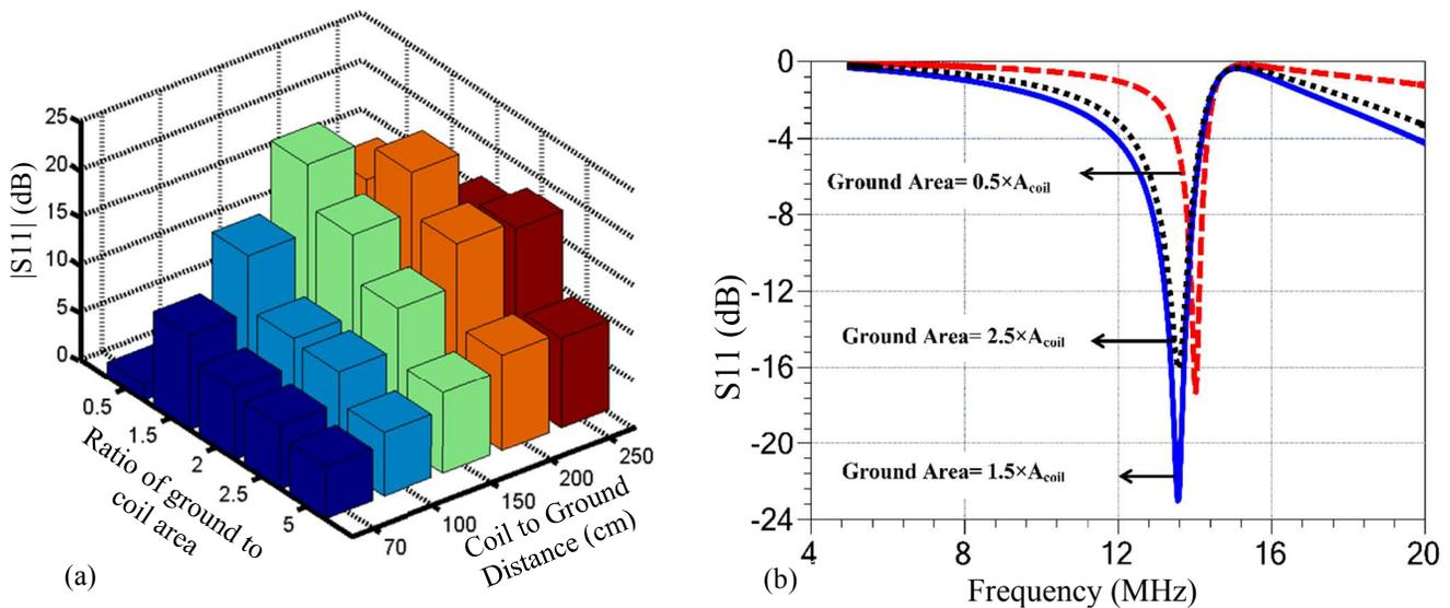
**Fig. 5.** (a) Resonant amplitude of  $S_{11}$  vs. ground to coil distance and ground to coil area ratio, (b)  $S_{11}$  profile for different areas of ground plane at the distance of 200 cm between the ground and coil
