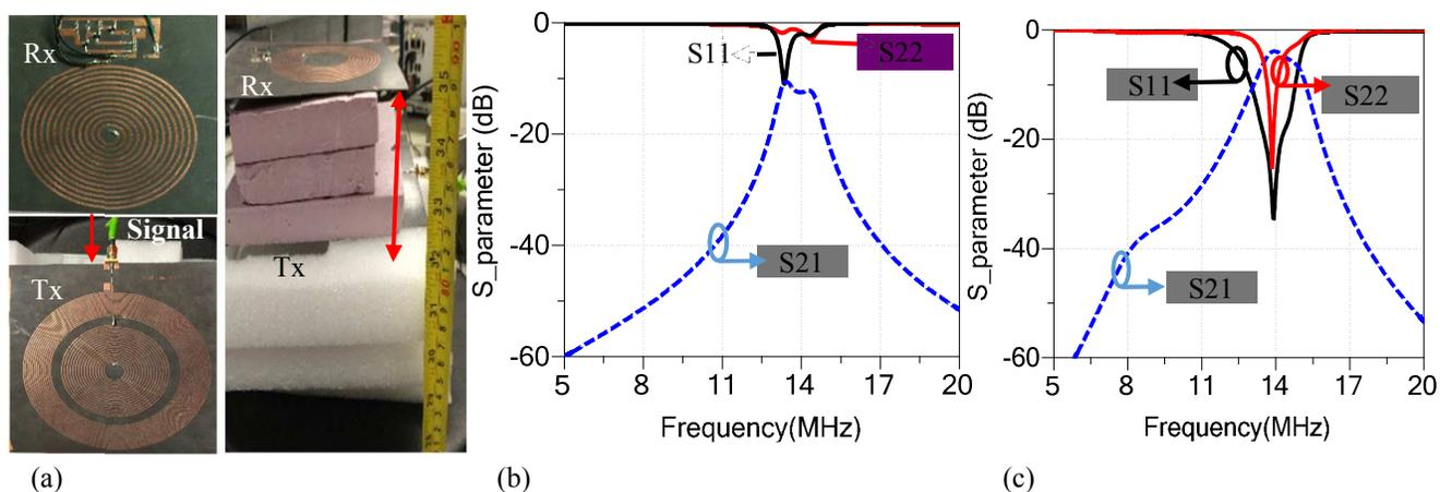
**Fig. 8.** (a) Implemented GE open-ended Tx coil and a conventional Rx coil with distance of 6 cm, the electrical ground plate is 79cm away from the Tx coil, (b) Measured S-parameters for open-ended Tx and conventional Rx resonant coils in unmatched condition, (c) S-parameter of the system in matched condition.
