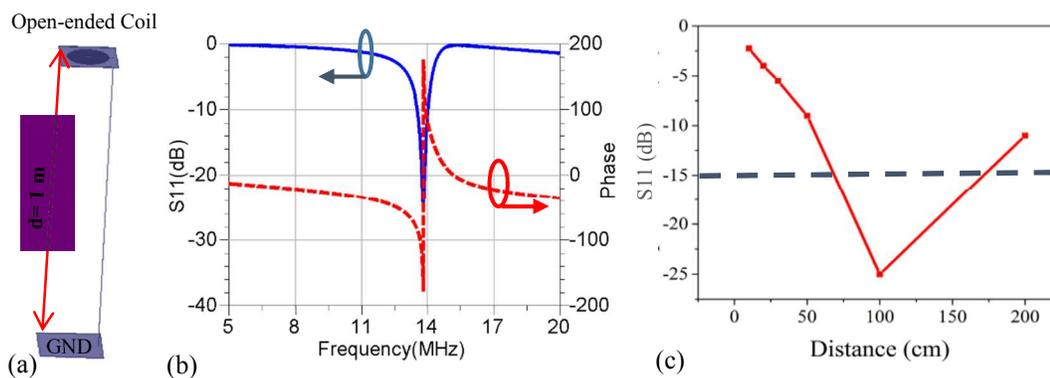
**Fig. 3.** (a) Open-ended resonator with single feed, (b) Simulation results of the  $S_{11}$  parameter with amplitude and phase at the resonant frequency, (c)  $S_{11}$  resonant amplitude for a variant distance between the ground and the coil plane at 13.5 MHz.
