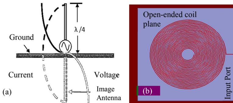
Fig. 2. (a) Marconi's antenna structure with a length of  $\lambda/4$ , (b) Implemented structure in HFSS with one feed line and one open-ended terminal. The ground plane is considered 100 cm below from the coil plane.
