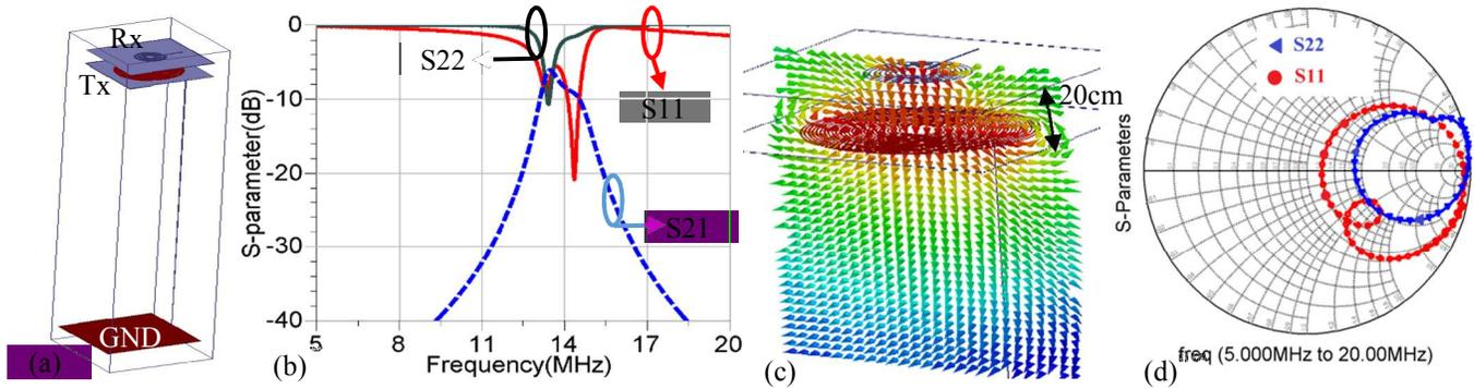
**Fig. 4.** (a) Simulated structure, conventional (Rx) Open-ended resonator(Tx), (b) S-parameter of the coupled coils, where  $S_{21}$  shows an acceptable level of transmitted power from Tx to Rx at operation frequency of 13.56 MHz, (c) Magnetic field in vector in between the coils and ground plane, (d) Smith chart of the coupled coils.
