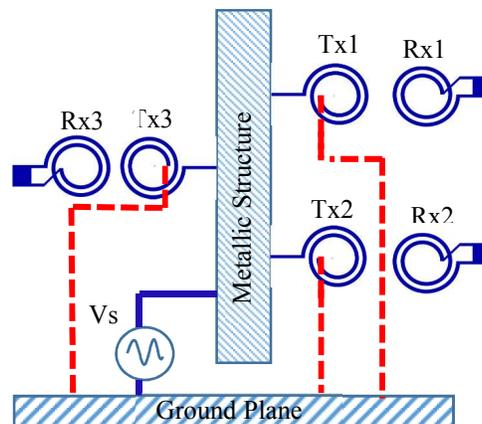
Fig. 1. Schematic of the proposed WPT system
