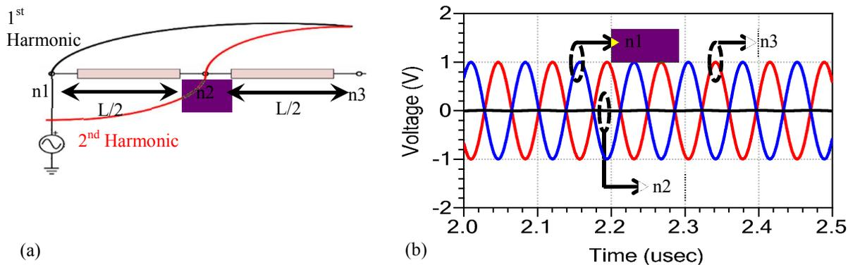
**Fig. 6.** (a) Open-ended resonator schematics and voltage propagation profile along the wire for the first and second harmonics, (b) Transient response of the voltage signal at the selected nodes on the coil trace.
