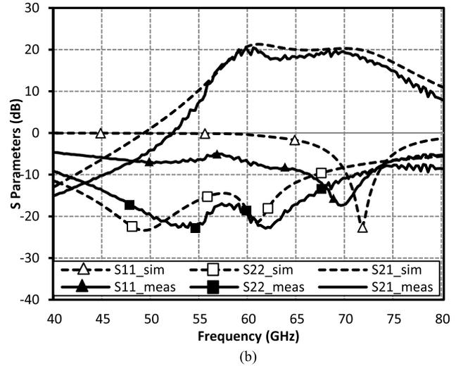
Fig. 11. Small-signal measurements and simulation results. (a) LP class A. (b) HP class AB dual mode.
