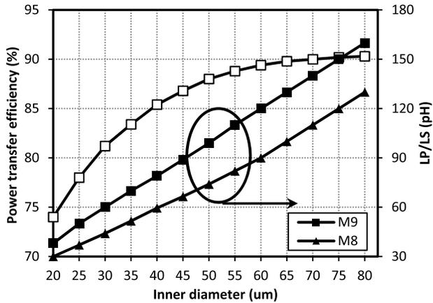
Fig. 6. EM simulation results for extracted inductance and efficiency of stacked transformers at 60 GHz respect to the size of the inner diameter.
