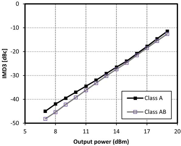
Fig. 14. Measured third-order intermodulation in class A and class AB.
