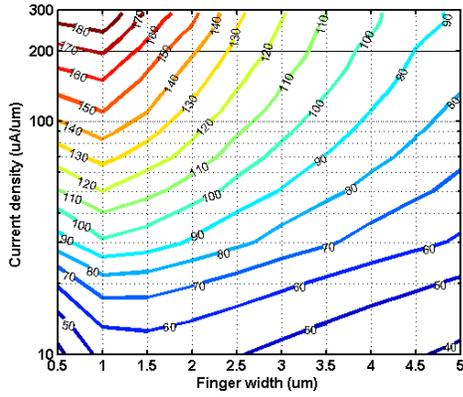
Fig. 2. Extracted  $f_{max}$  of dual-mode power stages from unilateral power gain, with respect to the total size of the stage. Devices are 30 numbers of fingers.
