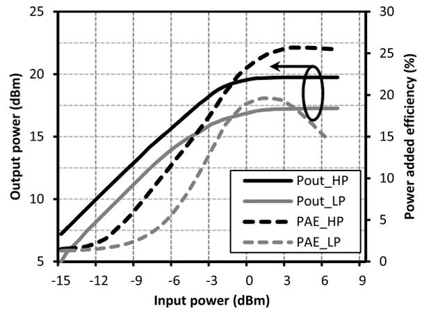
Fig. 13. Measured output power and PAE in HP and LP modes.
