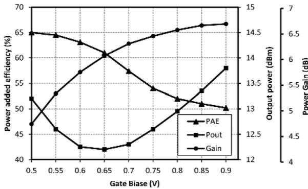
Fig. 3. Simulated maximum power gain, output power, and PAE of the dual-mode stage respect to the gate bias ( $V_G$ ).
