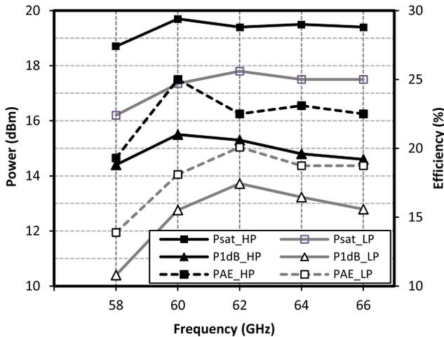
Fig. 15. Measured PA saturated output power,  $P_1$  dB, and PAE over the IEEE 802.15.3c band.
