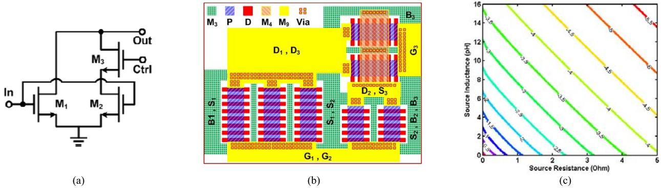
Fig. 1. Proposed dual-mode amplification. (a) Single-ended PA circuitry for illustration purpose. (b) Layout of the proposed topology. (c) Stage power gain degradation due to the parasitic source resistance and inductance added to all unit cells.
