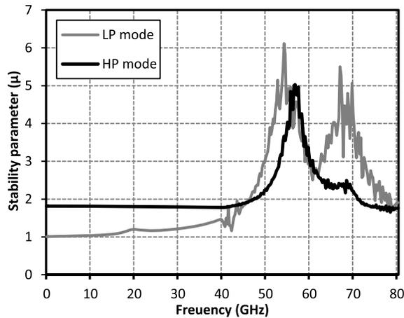
Fig. 12. Measured stability parameters for LP/HP modes.
