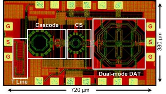
Fig. 10. Chip micrograph of fabricated 60-GHz PA.
