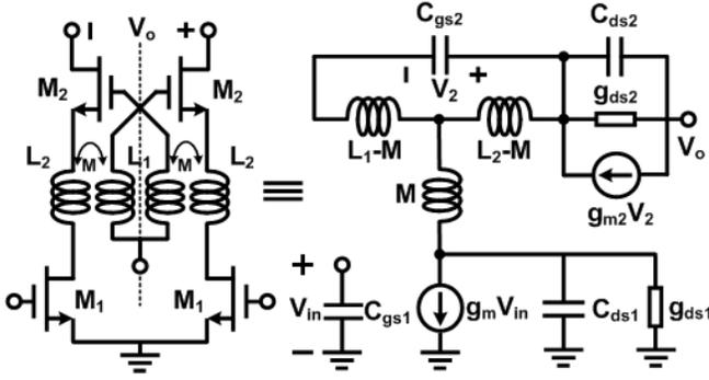
Fig. 8. Small-signal model of the gain-booster cascode stage.
