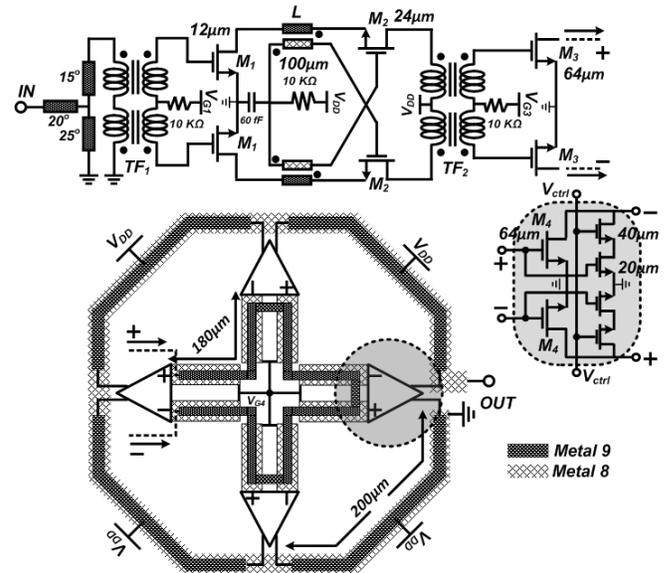
Fig. 5. Schematic and layout of three-stage 60-GHz differential DAT dual-mode PA.
