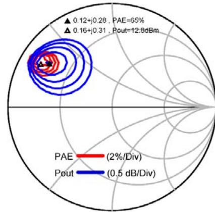
Fig. 4. Load-pull simulation of the proposed dual-mode stage ( $V_G = 0.75$ ).
