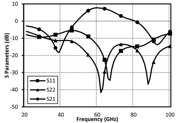
Fig. 7. Simulated S-parameters of the proposed dual-mode DAT.
