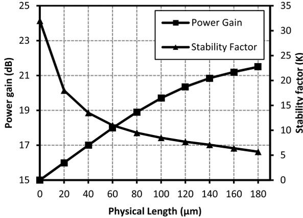
Fig. 9. Simulated power gain and stability factor of transformer-based neutralized cascode stage.
