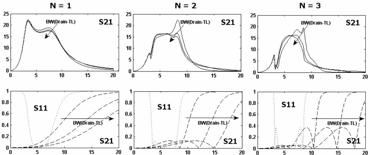
Fig. 4. S parameters simulation results for proposed bandpass DA with different number of stages ( $N=1, 2,$  and  $3$ ) and different bandwidth ratio of the drain and gate transmission line
