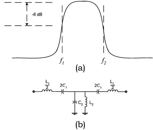
Fig. 3. a) Typical frequency response of bandpass LC filter, and b) its corresponding LC filter topology (single stage).
