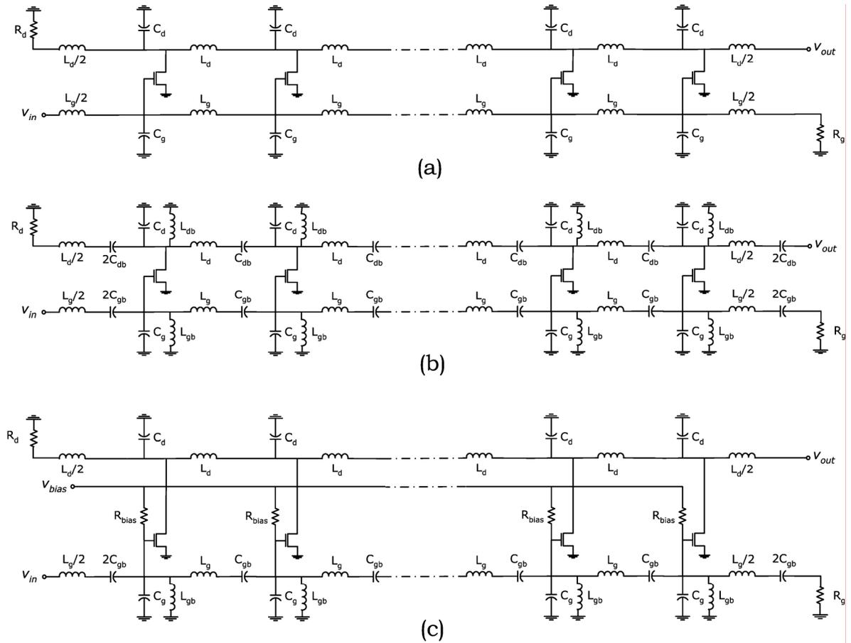
Fig. 2. Schematic diagrams of (a) conventional lowpass CMOS distributed amplifier, (b) bandpass CMOS distributed amplifier, and (c) modified bandpass CMOS distributed amplifier.
