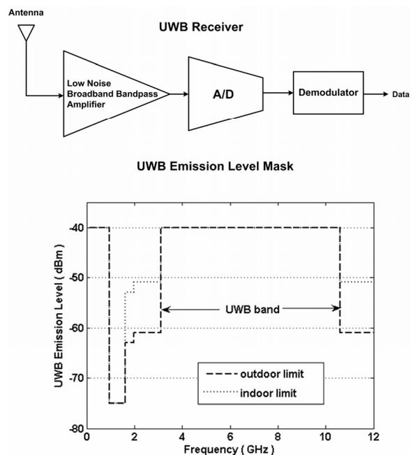
Fig.1. a) Block diagrams of UWB receivers, and (b) FCC's UWB emission mask.
