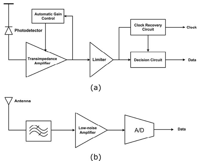
Fig. 1. (a) Block diagram of optical receivers, and (b) block diagram of UWB receivers
