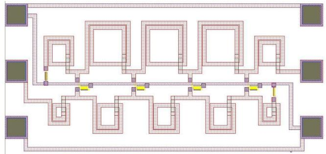
Fig. 6. Layout of the four-stage CMOS DA in 0.18  $\mu\text{m}$  CMOS technology with six metal layers.
