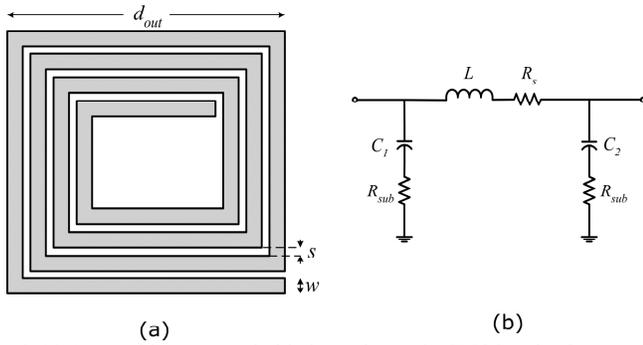
Fig. 4. (a) An on-chip square spiral inductor layout in CMOS technology, and (b) equivalent circuit of the on-chip square spiral inductor.
