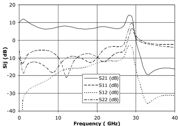
Fig. 5. S-parameter simulation results of the four-stage CMOS DA.
