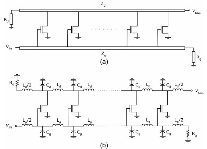
Fig. 3. (a) Schematic diagram of a uniform microwave distributed amplifier, and (b) schematic diagram of a uniform CMOS distributed amplifier constructed of artificial LC transmission lines.
