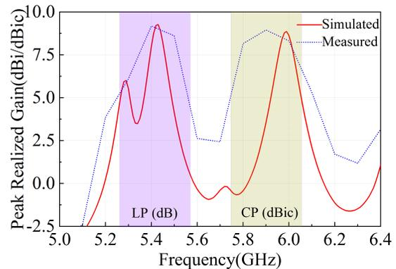
Fig. 11. Simulated and measured peak realized gain vs frequency
