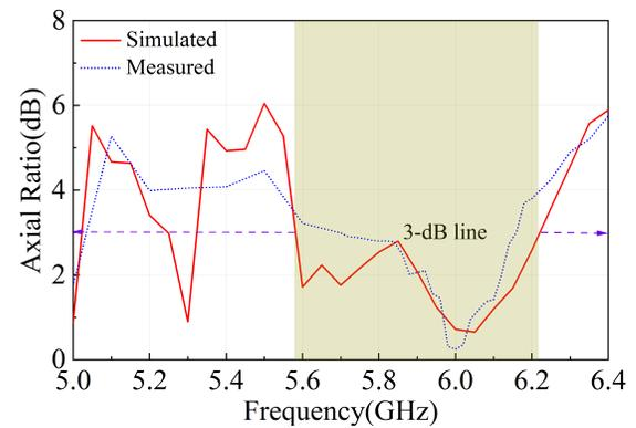
Fig. 10. Simulated and measured axial ratio of the proposed antenna.
