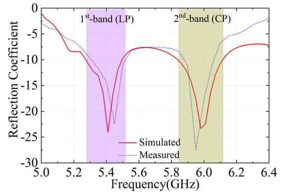
Fig. 9. Simulated and measured reflection coefficient.
