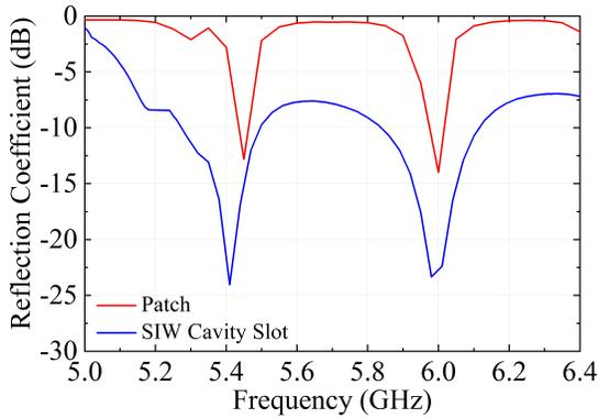
Fig. 6. Simulated reflection coefficient patch and SIW cavity slot antenna.
