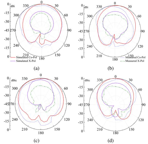
Fig. 13. Simulated and experimental normalized radiation pattern: (a) E-plane, (b) H-plane at  $f_1$  frequency, and (c) E-plane, (d) H-plane at  $f_2$ .
