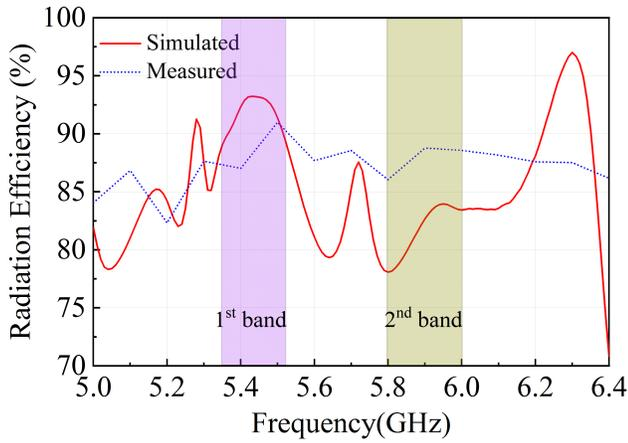
Fig. 12. Simulated and experimental plot of radiation efficiency.
