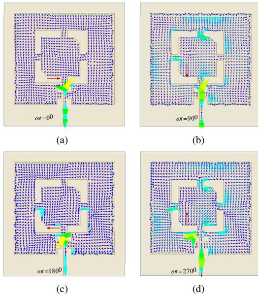
Fig. 7. Surface current distribution (vector) at 5.99 GHz: (a)  $\omega t = 0$  (b)  $\omega t = \frac{\pi}{2}$  (c)  $\omega t = \pi$  (d)  $\omega t = \frac{3\pi}{2}$ .
