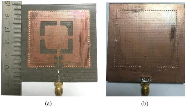
Fig. 8. Fabricated prototype of proposed antenna: (a) Top view and (b) bottom view.
