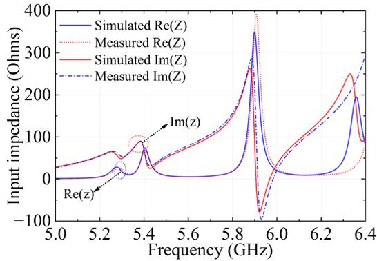
Fig. 5. Simulated input impedance vs frequency plot.
