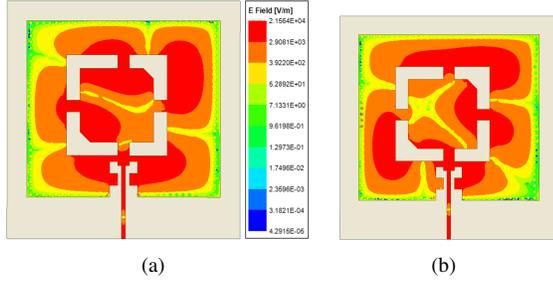
Fig. 4. Electric field distribution and different eigen mode of the SIW cavity: (a)  $TE_{201}$  and (b)  $TE_{202}$ .
