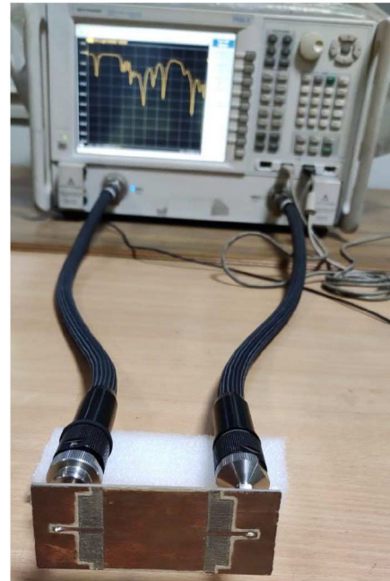
Fig. 6. The back-to-back transitions with VNA.
