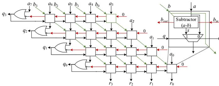
Fig. 18. An 8/4 unsigned restoring array divider.  $A = \sum_{i=0}^7 a_i 2^i$  and  $B = \sum_{i=0}^3 b_i 2^i$  are the input dividend and divisor, respectively.  $Q = \sum_{i=0}^3 q_i 2^i$  and  $R = \sum_{i=0}^3 r_i 2^i$  are the output quotient and remainder, respectively. The OR gate is a simplified subtractor with 0 as the subtrahend for dealing with overflow.
