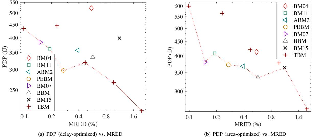
Fig. 17. A comparison of power-delay product and MRED for the approximate  $16 \times 16$  Booth multipliers.
