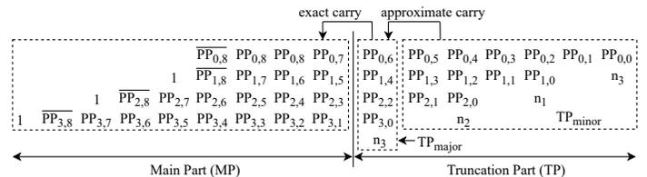
Fig. 14. The partial product (PP) partition for an  $8 \times 8$  fixed-width modified Booth multiplier [136].  $PP_{i,j}$  is the  $j^{\text{th}}$  PP in the  $i^{\text{th}}$  PP vector,  $\overline{PP}_{i,j}$  is the inverted  $PP_{i,j}$ , and  $n_i$  is the sign of the  $i^{\text{th}}$  encoded digit.
