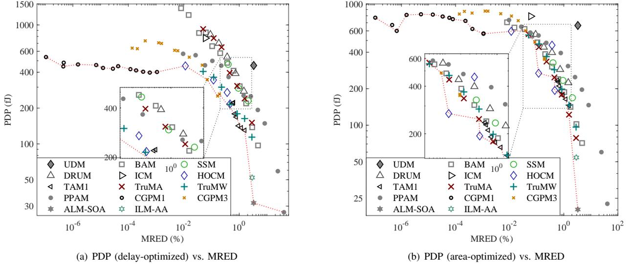
Fig. 13. A comparison of power-delay product and MRED for the approximate  $16 \times 16$  unsigned multipliers.
