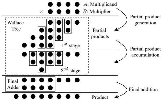
Fig. 9. The basic arithmetic process of a  $4 \times 4$  unsigned multiplication.  $\bullet$ : an input, a partial product or an output bit;  $\square$ : a half adder, a full adder or a 4:2 compressor.
