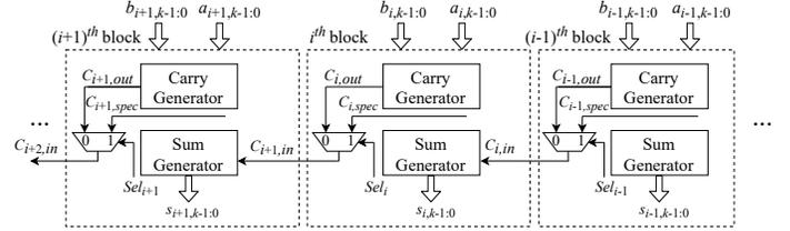
Fig. 4. The approximate carry-select adder with carry-in selection.
