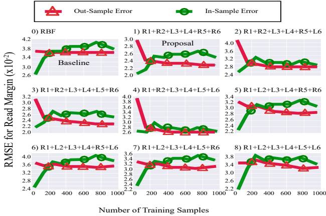
Fig. 3: Mean out-sample prediction error and mean in-sample error for dynamic read margin modeling of 6T SRAM at 0.3V for 20 iterations of GP regression. The proposed model has the minimum out-sample error. (R = RBF kernel and L = Linear kernel)
