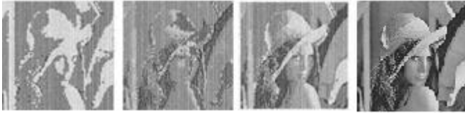
Fig. 18. The progressive improvement of image quality using squared L^2 -norm stochastic VQ after 256, 512, 1024 and 2048 clock cycles.
