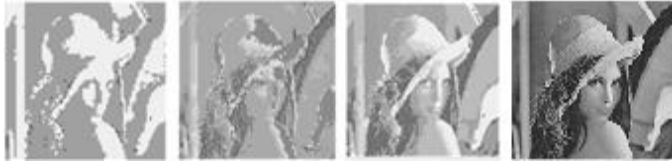
Fig. 19. The progressive improvement of image quality using the 3^{rd} -law stochastic VQ after 256, 512, 1024 and 2048 clock cycles.
