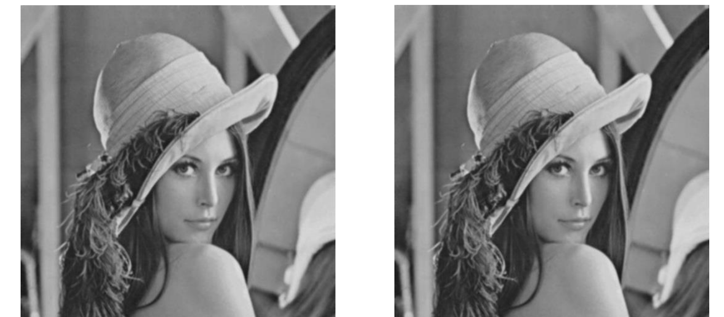
Fig. 7 Image smoothing results using an approximate multiplier (left) and an accurate multiplier (right)
