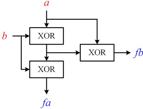
Fig. 7. Eliminating wire crossing using XOR gates in [20].
