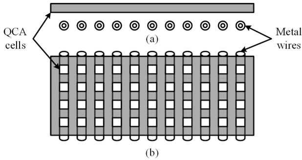
Fig. 3. Metal wires for providing electric field (a) Front view (b) Top view.
