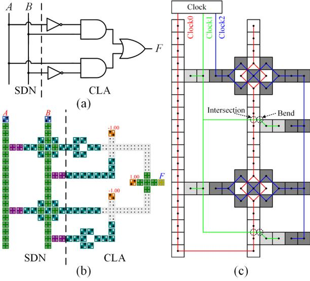
Fig. 9. An XOR gate (a) Diagram in [28] (b) Implementation in QCA using the proposed SDN (c) Circuitry of metal wires for the SDN in an XOR.
