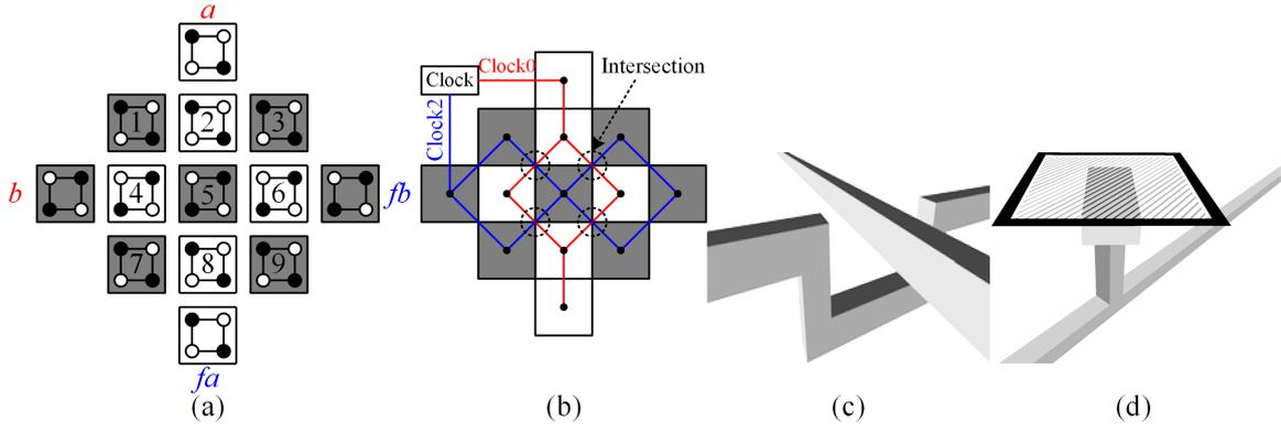
Fig. 8. Proposed wire crossing (a) Layout (b) Circuitry of metal wires (c) Metal wire crossing (d) Metal pad.
