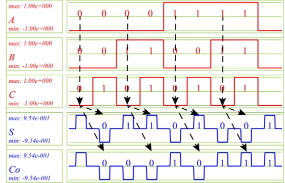
Fig. 13. Simulation results for a full adder using the proposed SDN.
