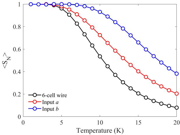
**Fig. 16.** Thermal characteristics for a 6-cell wire and two signal transmission branches in the proposed wire crossing.**Table 6**
