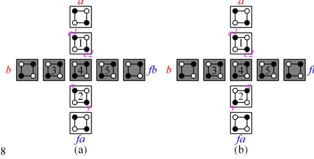
Fig. 15. Different electron arrangements for the wire crossing in [24] (a) Case 1 (b) Case 2.
