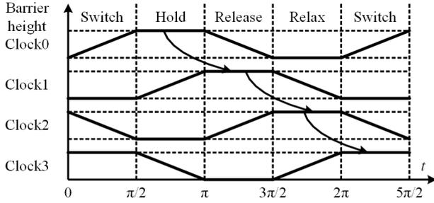
Fig. 2. QCA four-phase clock mechanism.
