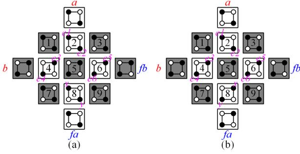
Fig. 14. Different electron arrangements for the proposed wire crossing (a) Case 1 (b) Case 2.
