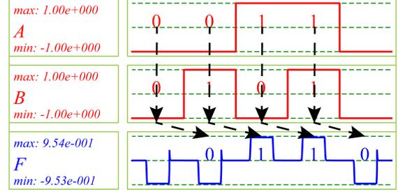
Fig. 12. Simulation results for an XOR gate using the proposed SDN.
