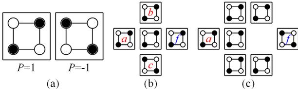
Fig. 1. QCA basics (a) QCA cells (b) Majority voter (c) Inverter.
