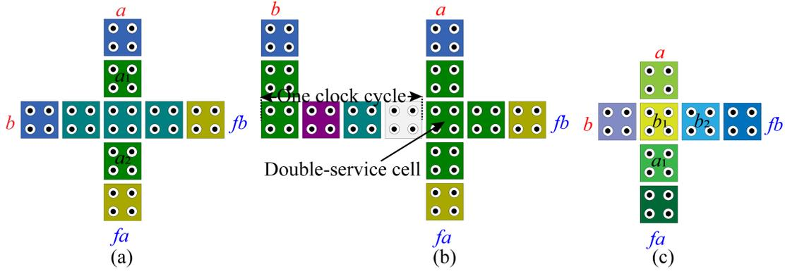
Fig. 5. Coplanar wire crossing using clock signals (a) Two signals in [24] (b) Four signals in [28] (c) Seven signals in [25].
