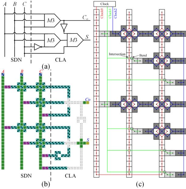
Fig. 10. A full adder (a) Diagram in [28] (b) Implementation in QCA using the proposed SDN (c) Circuitry of metal wires for the SDN in a full adder.
