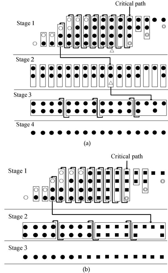
Fig. 2 The  $8 \times 8$  Booth multiplier using: (a) exact irregular partial product array, (b) approximate regular partial product array by ignoring the Neg term in the 5th partial product row. (The exact partial product term is represented by  $\bullet$ , while the approximate partial product term is represented by  $\blacksquare$ .  $\circ$  and  $\odot$  represent the sign extension bit and the Neg term.)
