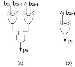
Fig. 1. The gate-level circuit of: (a) R4ABE1 and (b) R4ABE2.
