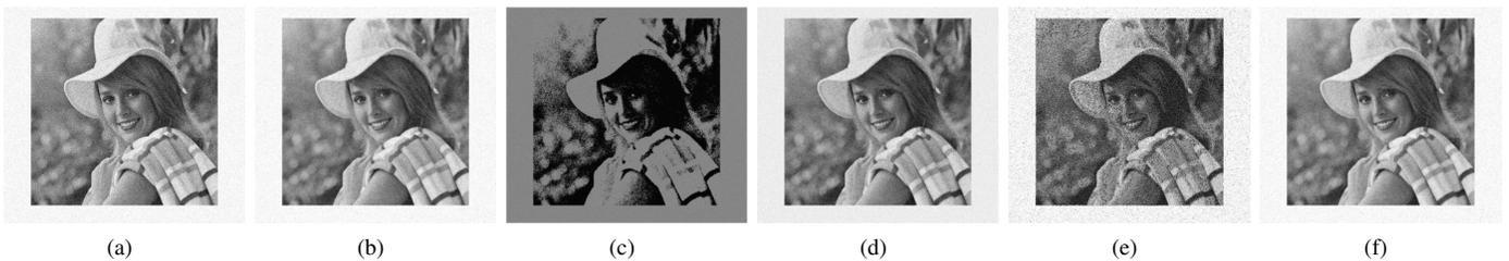
Fig. 13. Arithmetic mean filter: (a) original image with noise, (b) using exact adders, (c) using the ESA with  $k=5$  and  $PSNR=10.5dB$ , (d) using the ESA with  $k=8$  and  $PSNR=27.2dB$ , (e) using the ETAII with  $k=3$  and  $PSNR=16.9dB$  and (f) using the ETAII with  $k=5$  and  $PSNR=36.3dB$ .
