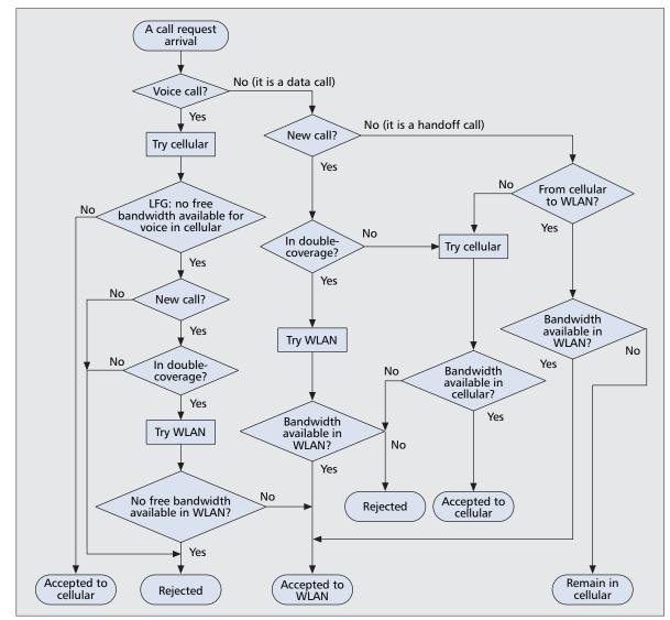
■ Figure 3. Call admission procedure for cellular/WLAN interworking.
