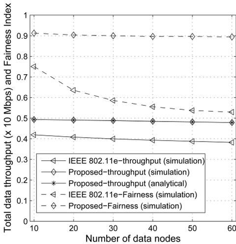
Fig. 7. The total data throughput and Fairness Index versus the number of data nodes in a fully connected network with only data traffic.
