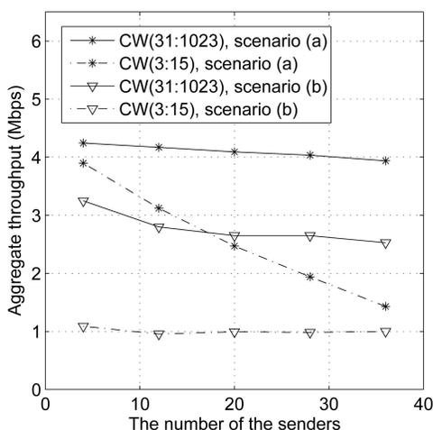
Fig. 11. The aggregate throughput versus the number of senders for IEEE 802.11e with different CW settings.
