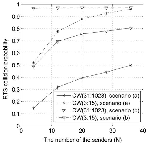
Fig. 10. The RTS collision probability versus the number of senders for IEEE 802.11e with different CW settings.
