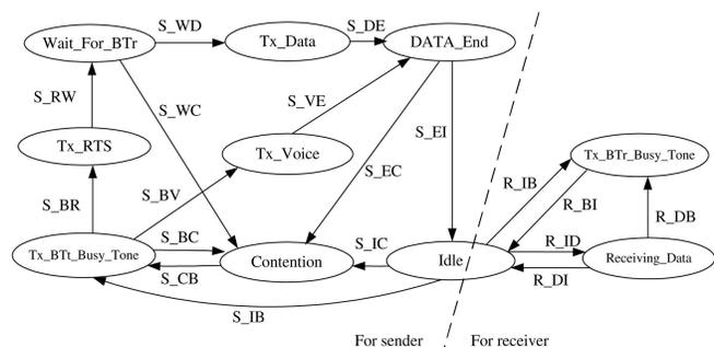
Fig. 9. The state transition diagram of the proposed scheme.
