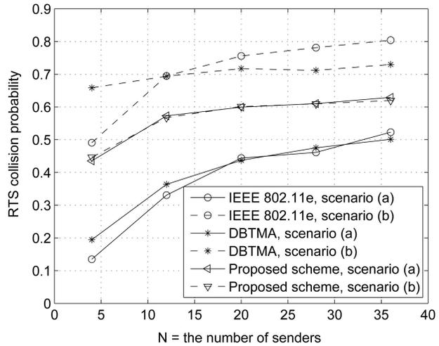
Fig. 4. RTS collision probability for IEEE 802.11e, DBTMA, and our scheme in scenarios (a) and (b).
