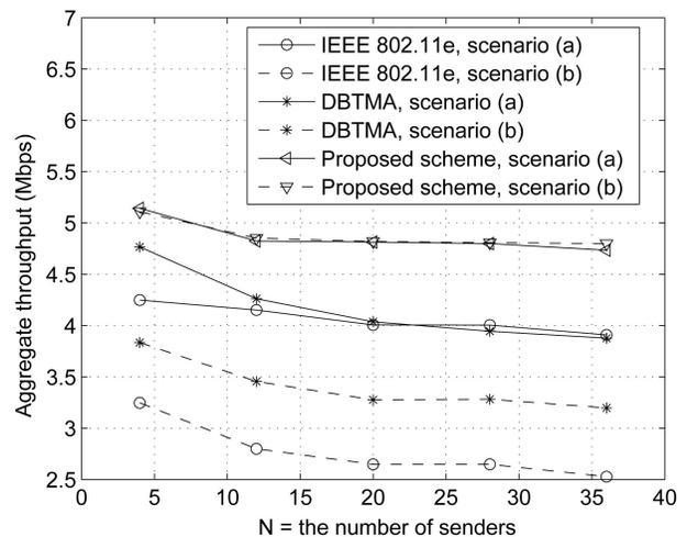
Fig. 5. The aggregate throughput of IEEE 802.11e, DBTMA, and proposed scheme in scenarios (a) and (b).
