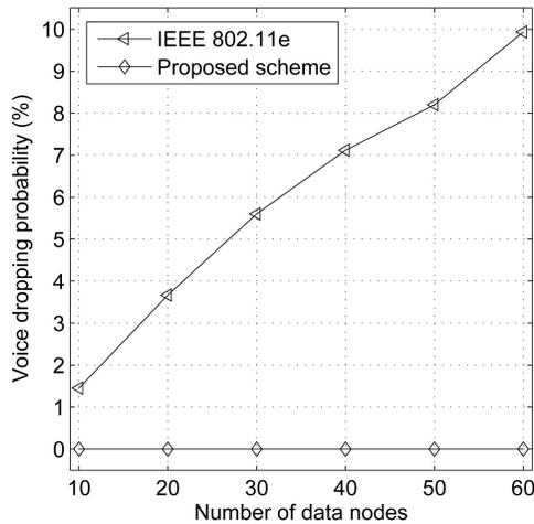
Fig. 6. Voice frame dropping probability versus the number of data nodes in a fully connected network with 20 voice nodes.
