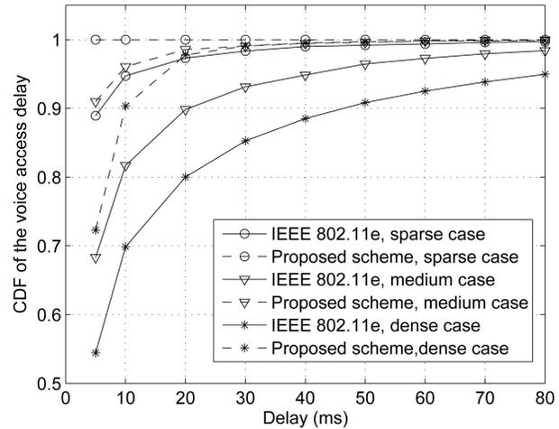
Fig. 8. The CDF of voice access delay in random topologies.
